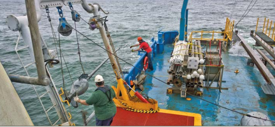
Piston coring of shallow sediments off the shore of San Luis Pass, Texas. Seismic and geochemical indications of natural-gas migration at the site have implications for long-term retention of carbon dioxide.
