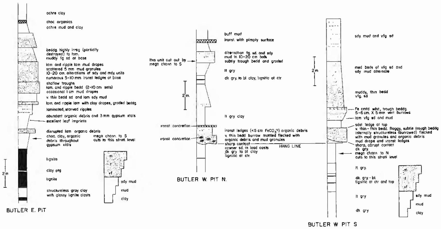
Figure 6. Graphic measured sections at Butler, Texas. At left, east pit (east of FM 696); middle and right, west pit (west of FM 696).
