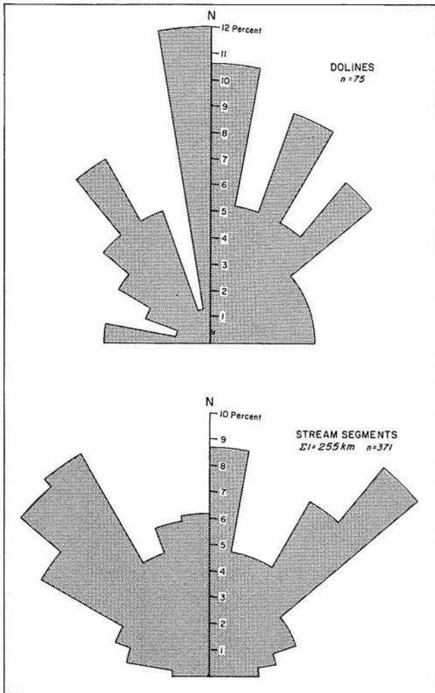
Figure 17. Diagrams indicating orientations of long axes of dolines and linear stream segments in Hall County, Texas. For each 10° sector, linear data are plotted as a percentage of the total number of closed depressions and as a percentage of total length of linear stream segments.
