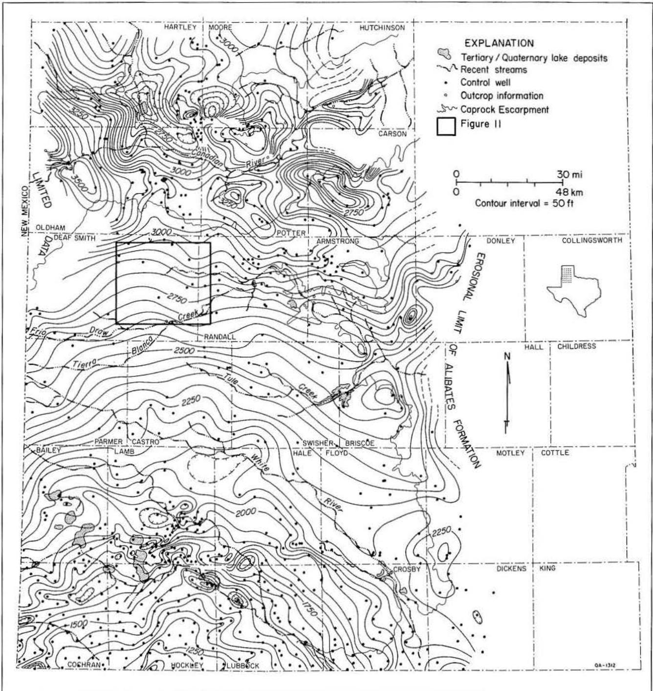
Figure 9. Structure-contour map on the top of the Alibates Formation. Note that structures are complex and well defined in areas of sufficient data but show little structural detail in areas of sparse data.
