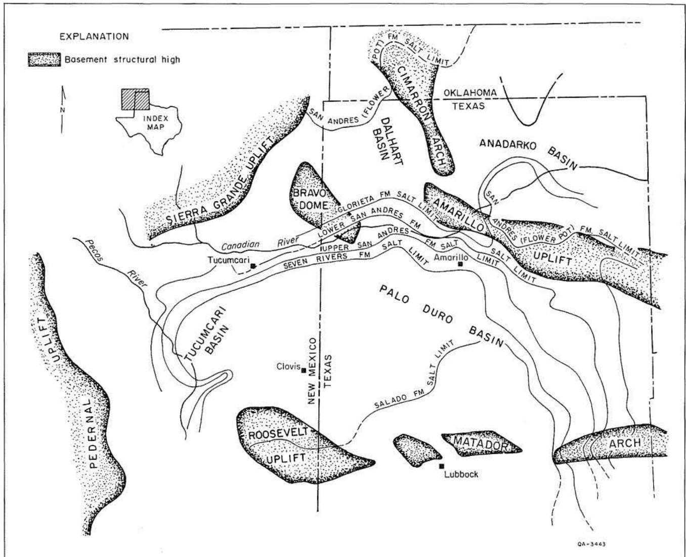
Figure 1. Major structural elements, Texas Panhandle and surrounding areas (after Nicholson, 1960). Limits of Permian bedded salts are closely associated with the structural margins of the Palo Duro Basin. Structurally high salt units are most likely to be affected by dissolution.
