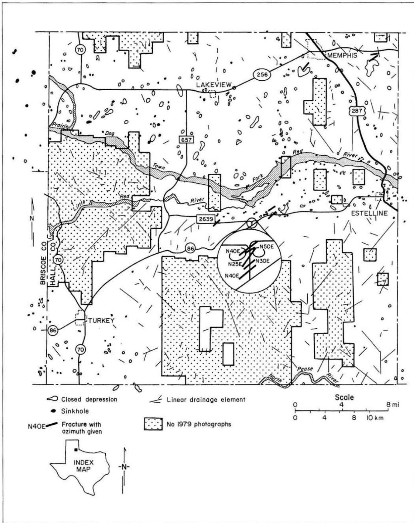
Figure 16. Location of sinkholes, closed depressions (dolines), and fractures in Hall and eastern Briscoe Counties, Texas. Dolines are drawn to scale; sinkholes, which are much smaller, are not drawn to scale. Dolines and sinkholes were recognized from color aerial photographs taken in 1979.
