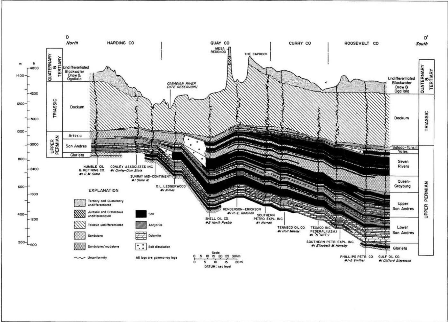
Figure 5. Stratigraphic cross section illustrating salt dissolution and collapse of strata beneath the Canadian River. See figure 3 for the location of section D-D'.
