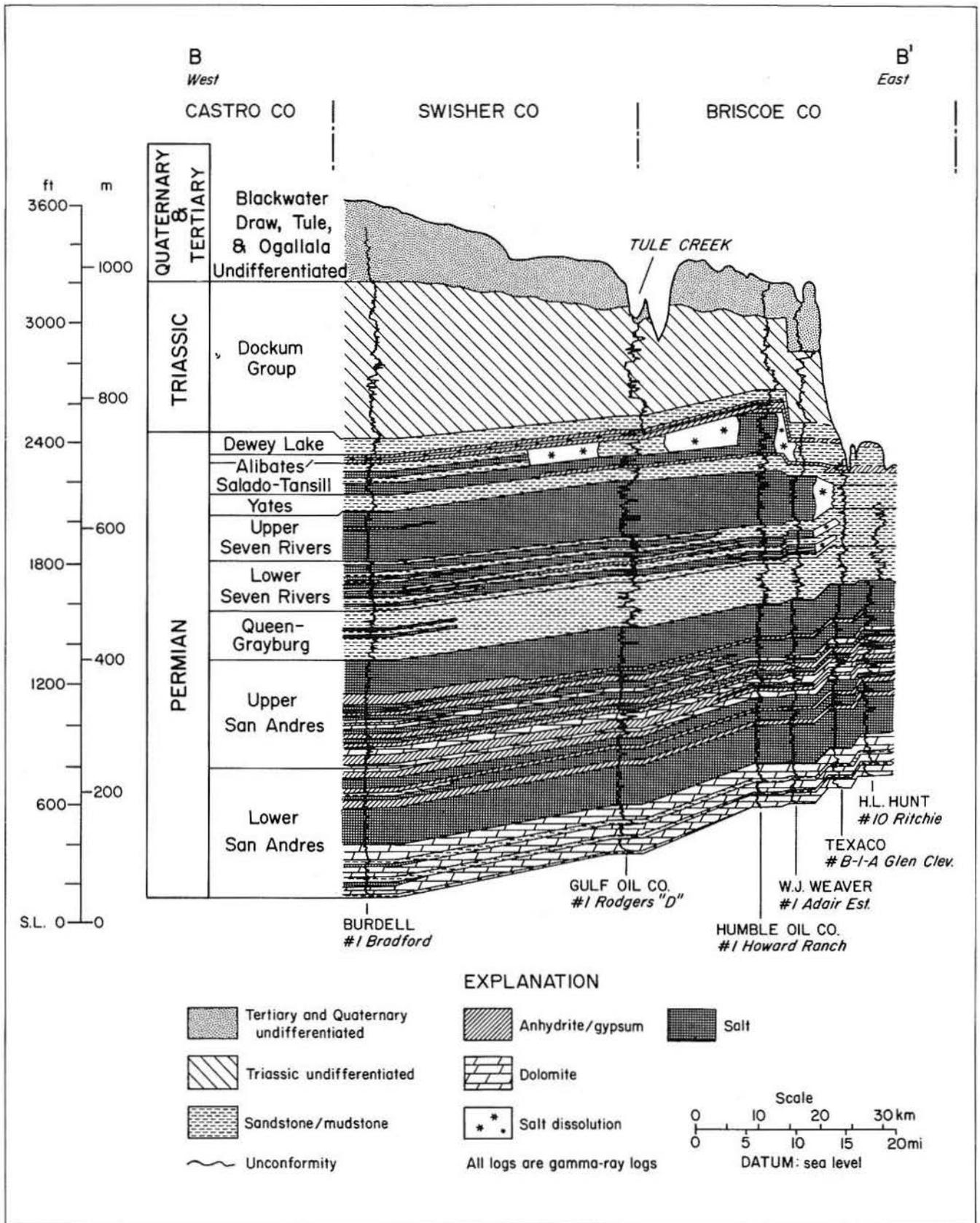
Figure 6. Stratigraphic cross section illustrating salt dissolution and collapse of overlying strata beneath Tule Creek. Tule Formation lacustrine beds, not shown on the cross section, crop out along the valley sides of Tule Creek. See figure 3 for the location of section B-B'.
