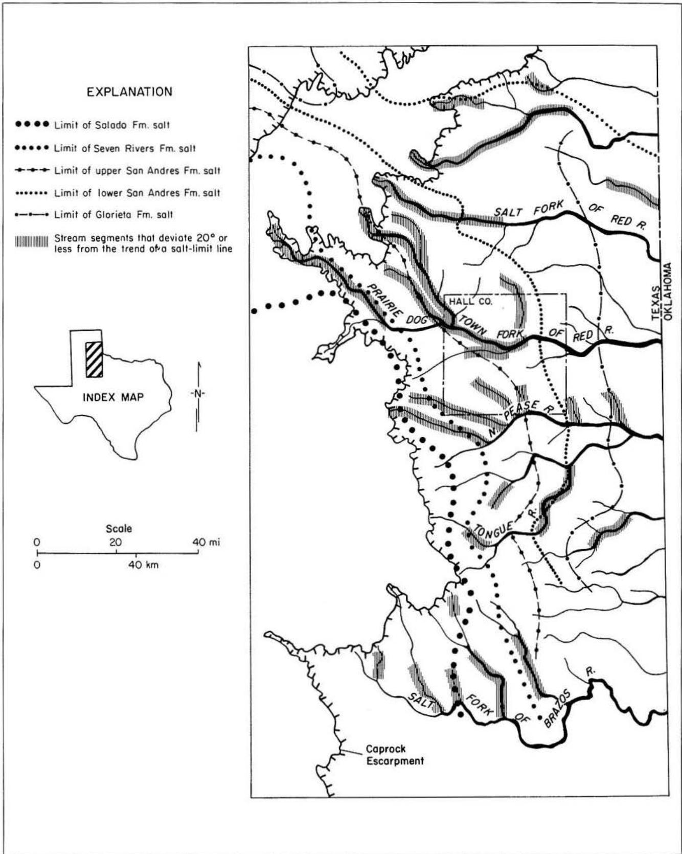
Figure 20. Comparison of stream segments to trends of the eastern limits of Permian salts. Approximately 40 percent of the total length of major streams within the Rolling Plains of the Texas Panhandle lies within 20° of the orientation of one or more of these salt limits. For comparison, a random stream pattern would yield a value of only 22 percent.
