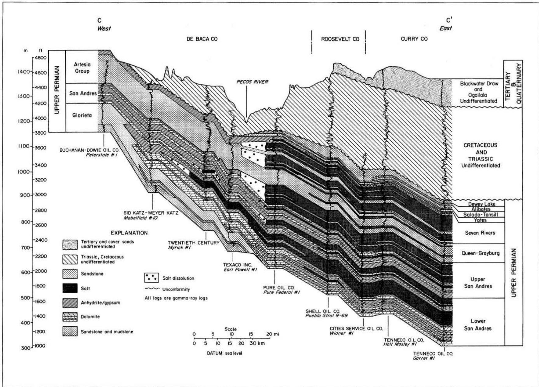
Figure 4. Stratigraphic cross section illustrating salt dissolution and collapse of strata beneath the Pecos River. See figure 3 for the location of section C-C'.
