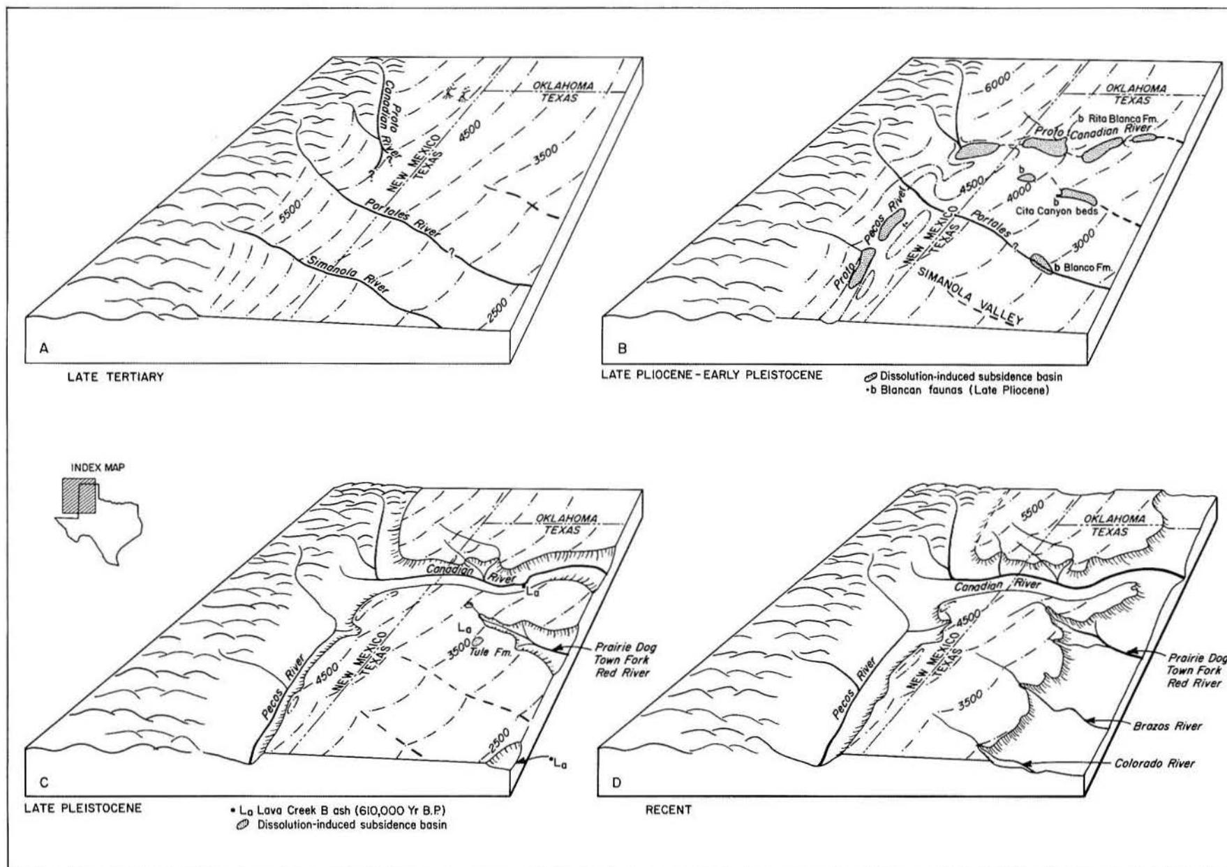
Figure 15. Evolution of drainage of eastern New Mexico and the Texas and Oklahoma Panhandles since the end of Ogallala deposition. Sizes of dissolution-induced subsidence basins are speculative because only remnants of these features were preserved. Rather than a few large basins, there may have been numerous small basins.
