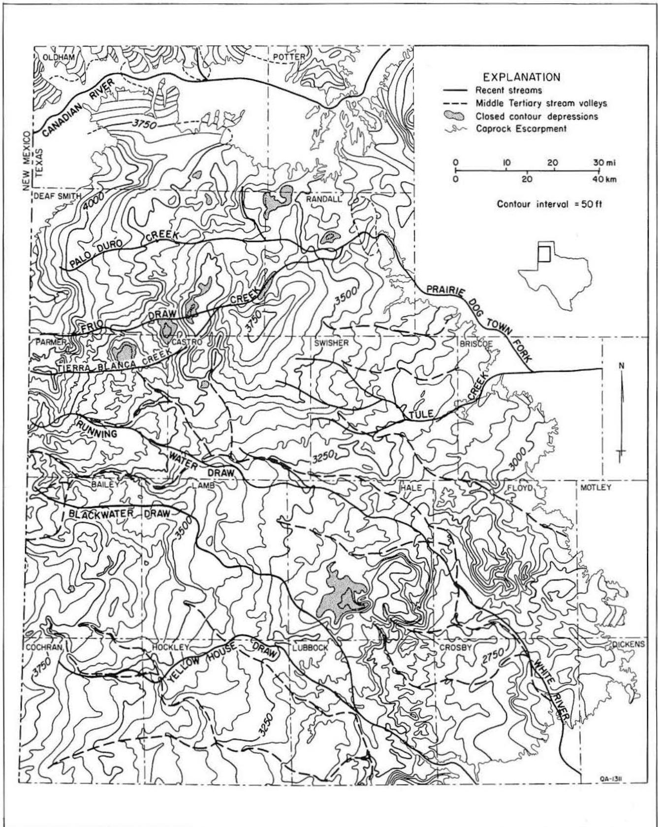
Figure 10. Structure-contour, or paleotopographic, map on the base of the Ogallala Formation (derived from Knowles and others, 1982). Paleostreams are interpreted from contour V's pointing upslope. Modern drainage is superimposed to show the relation between modern drainage and structure and between modern drainage and paleodrainage.
