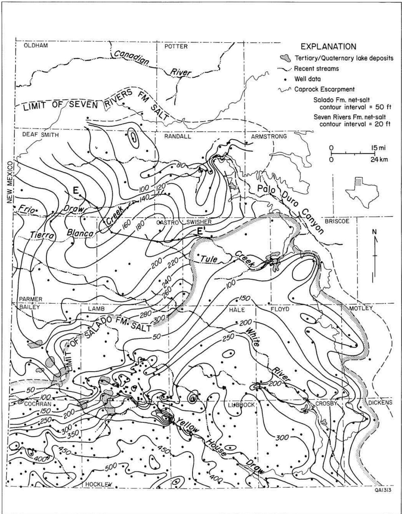
Figure 8. Net-salt map of parts of the Salado and Seven Rivers Formations. Net-salt thickness of the Seven Rivers Formation is shown only where Seven Rivers salts are not overlain by salts of the Salado Formation. Adapted in part from Gustavson and others (1981b).
