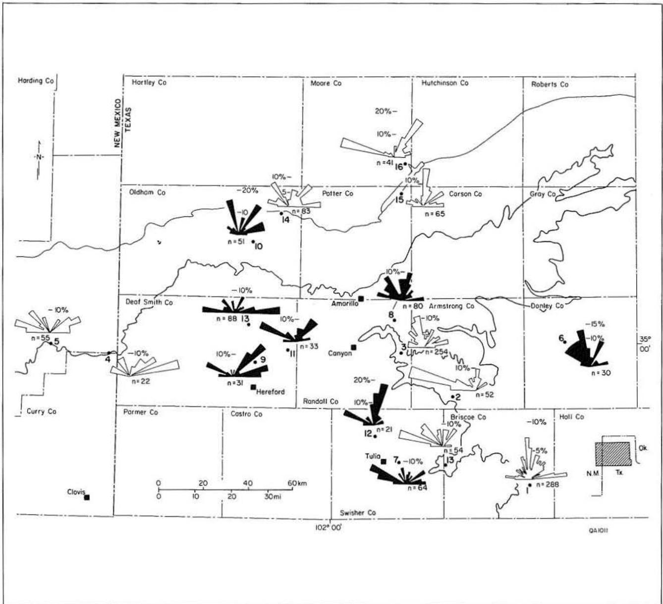
Figure 18. Fracture orientations from nine surface locations (open roses) in the Texas Panhandle and eastern New Mexico and from Schlumberger Fracture Identification Logs from eight test wells (filled roses) in the Texas Panhandle.
