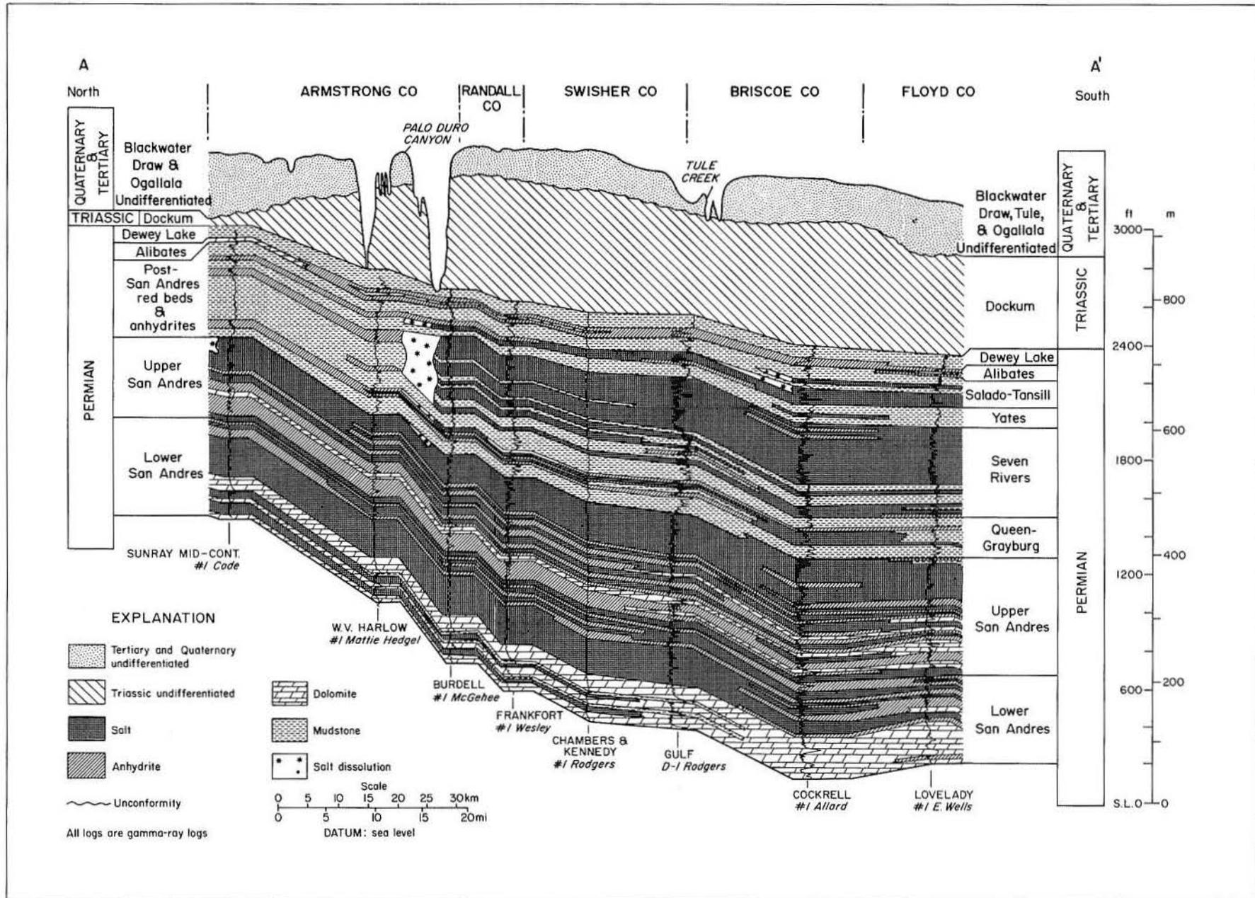
Figure 7. Stratigraphic cross section illustrating salt dissolution and collapse of overlying strata beneath the Palo Duro Canyon (Prairie Dog Town Fork of the Red River). See figure 3 for the location of section A-A'.
