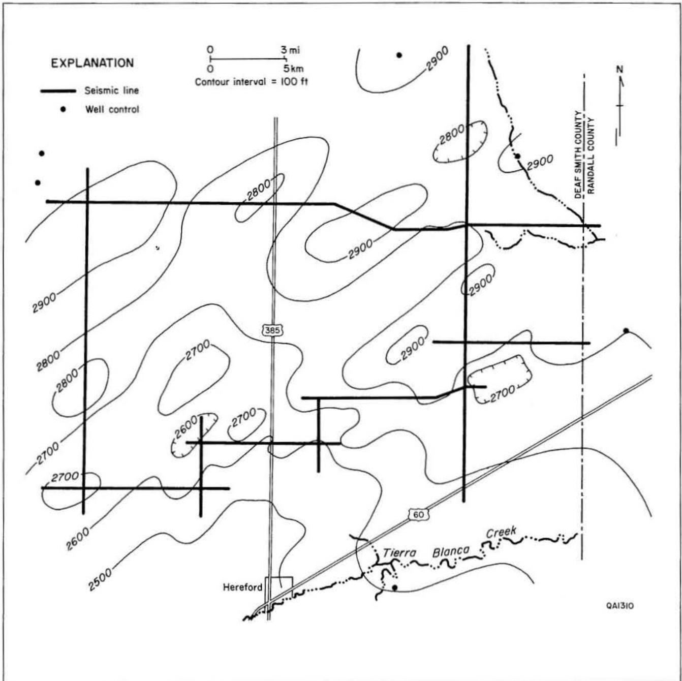
Figure 11. Structure-contour map on the top of the Alibates Formation, interpreted from seismic reflection velocity data. See figure 9 for location.
