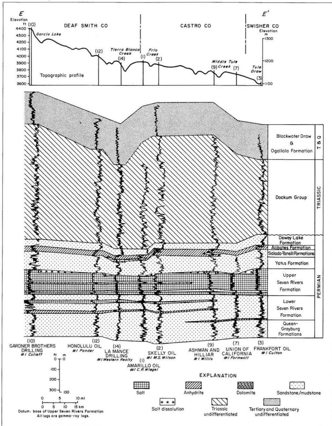
Figure 12. Stratigraphic section showing dissolution of Seven Rivers Formation salts and collapse of overlying strata beneath Tierra Blanca Creek (datum is base of the Seven Rivers Formation). See figure 8 for the location of section E-E'.
