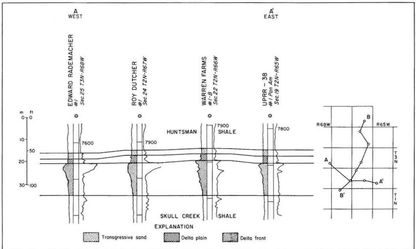
FIGURE 70. East-west stratigraphic cross section A-A' showing facies of the "J" Sandstone, Denver Basin (after Peterson and Janes, 1978).
