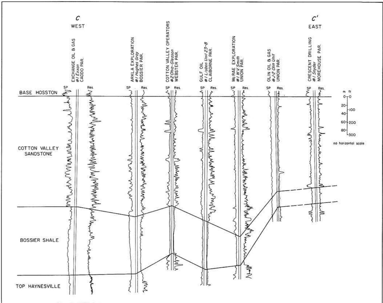
**FIGURE 39.** East-west stratigraphic cross section C-C' through the Cotton Valley Sandstone and underlying units, North Louisiana Basin (from Louisiana Office of Conservation, 1981). Line of section shown in figure 36.
