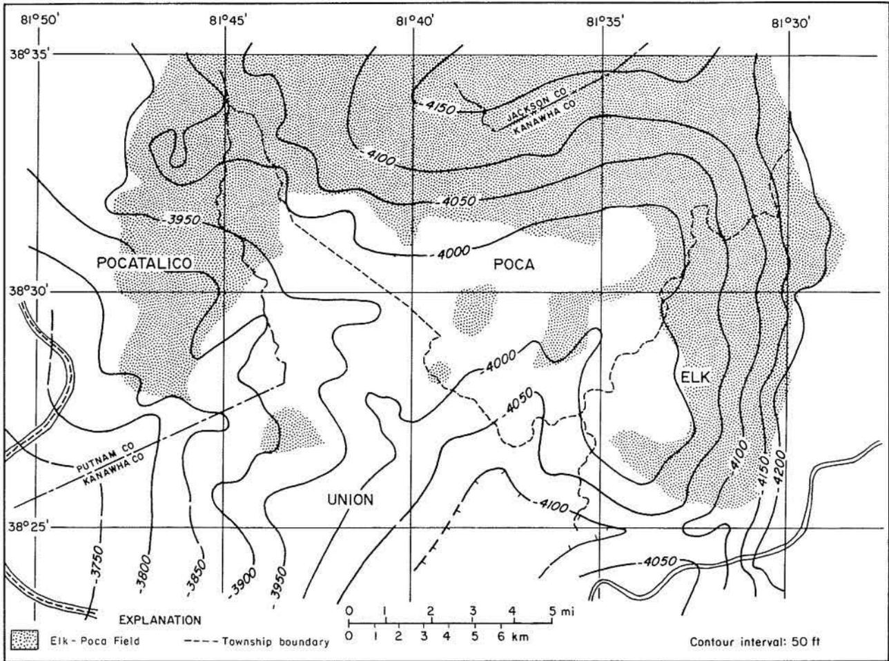
**FIGURE 10.** Structure contours on top of the Onondaga Limestone, Elk-Poca Field, South Sissonville area, West Virginia (from Diecchio, 1982b).
