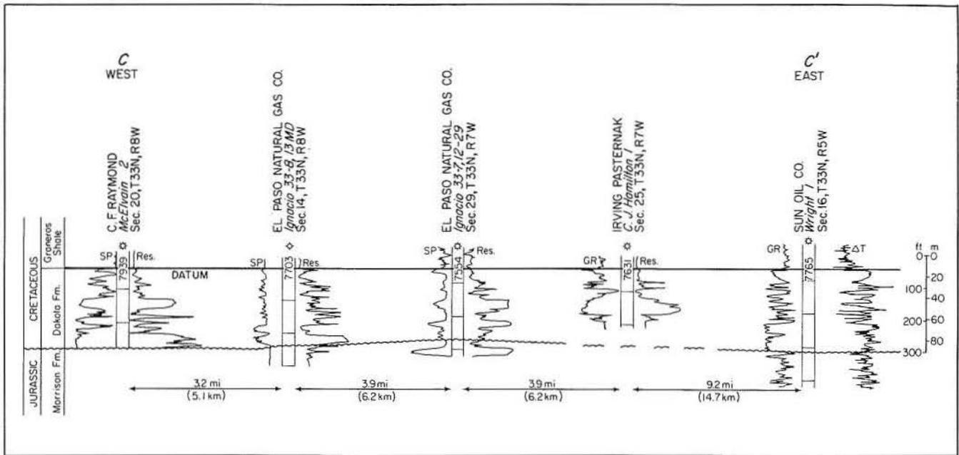
FIGURE 65. East-west stratigraphic cross section C-C through the Dakota Sandstone, San Juan Basin (after Colorado Oil and Gas Conservation Commission, 1981b). Line of section shown in figure 62.
