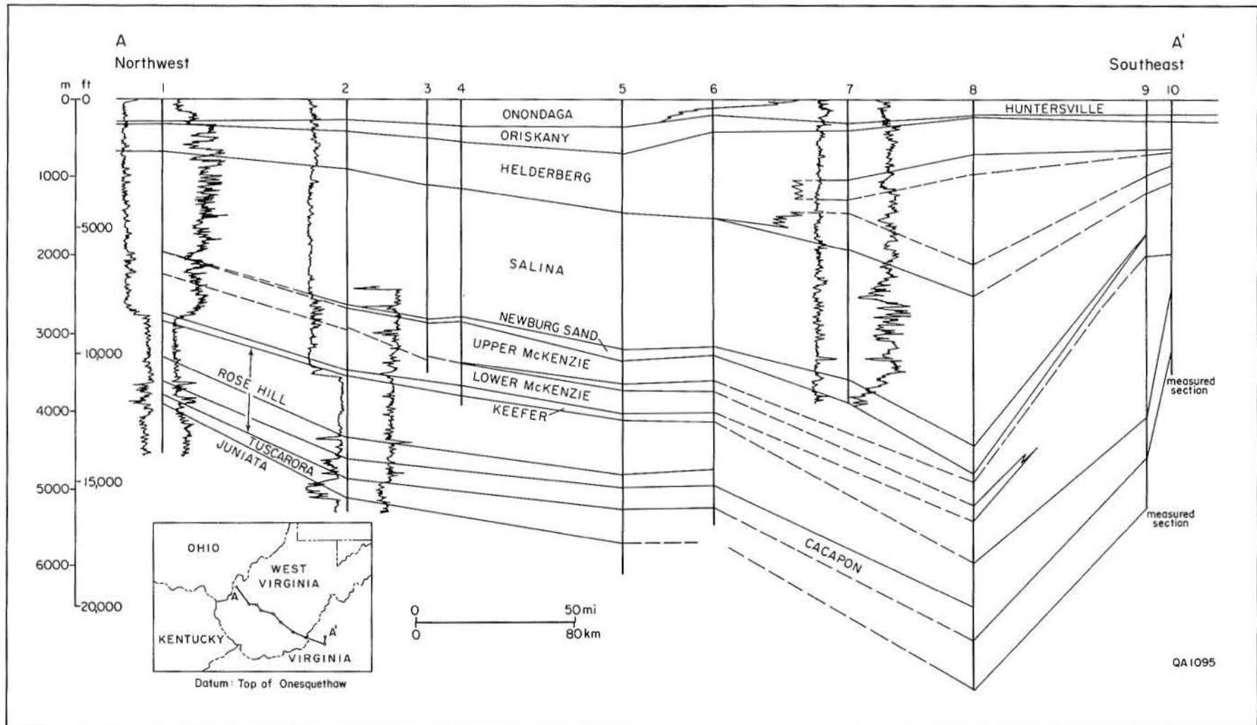
**FIGURE 15.** Northwest-southeast stratigraphic cross section A-A' through the Tuscarora Sandstone and overlying units showing thinning of the Tuscarora to the west (from Diecchio, 1982c; after Dennison, 1970).
