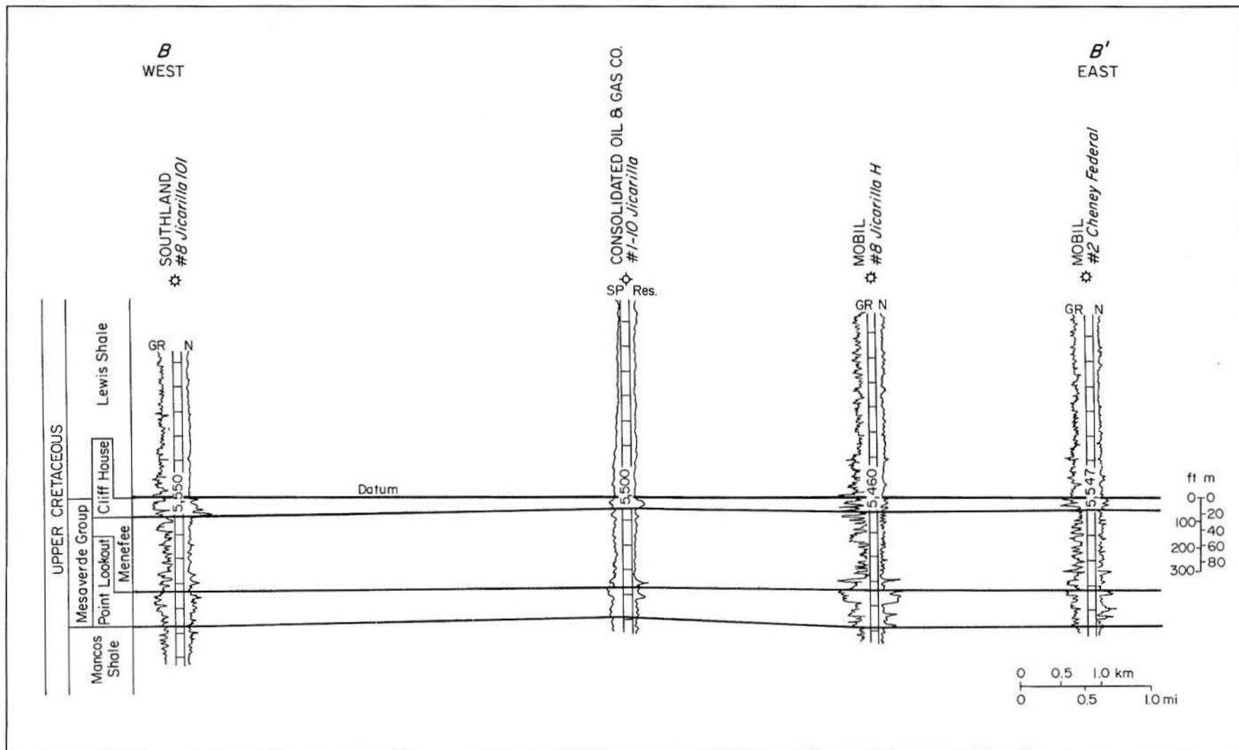
FIGURE 64. East-west stratigraphic cross section B-B' through the Mesaverde Group, San Juan Basin (after New Mexico Oil Conservation Division, 1981c). Line of section shown in figure 62.
