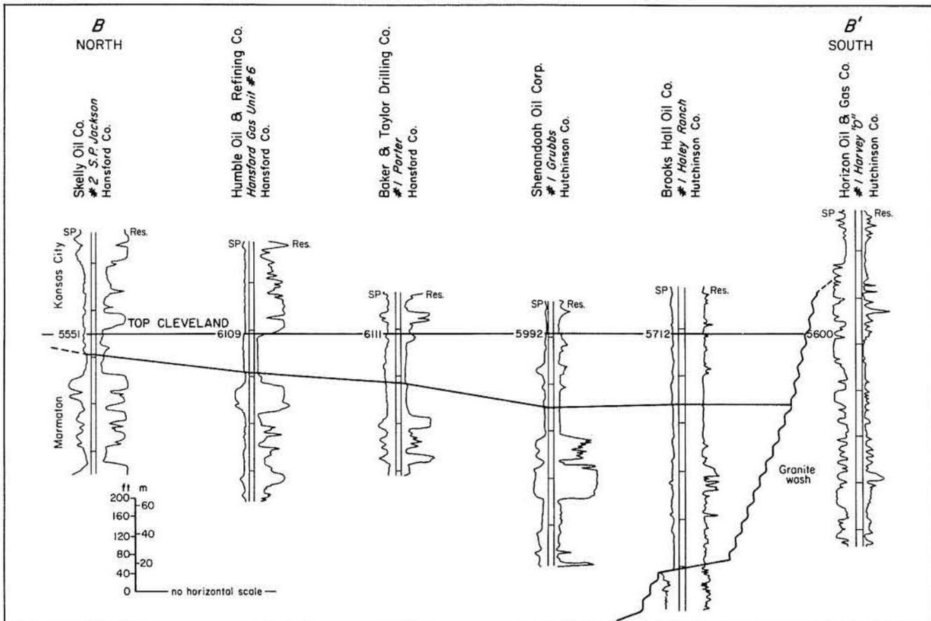
FIGURE 45. North-south stratigraphic cross section B-B' through the Cleveland Formation, Anadarko Basin (from Railroad Commission of Texas, 1981d). Line of section shown in figure 44.
