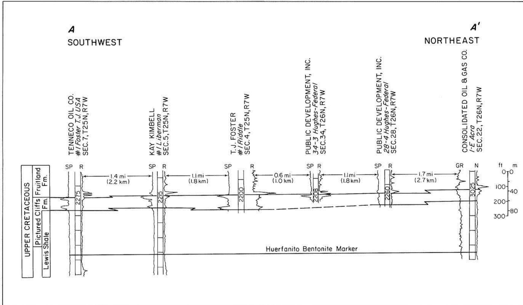
FIGURE 63. Northeast-southwest stratigraphic cross section A-A' through the Pictured Cliffs Sandstone and adjacent strata, San Juan Basin (after New Mexico Oil Conservation Division, 1982). Line of section shown in figure 62.
