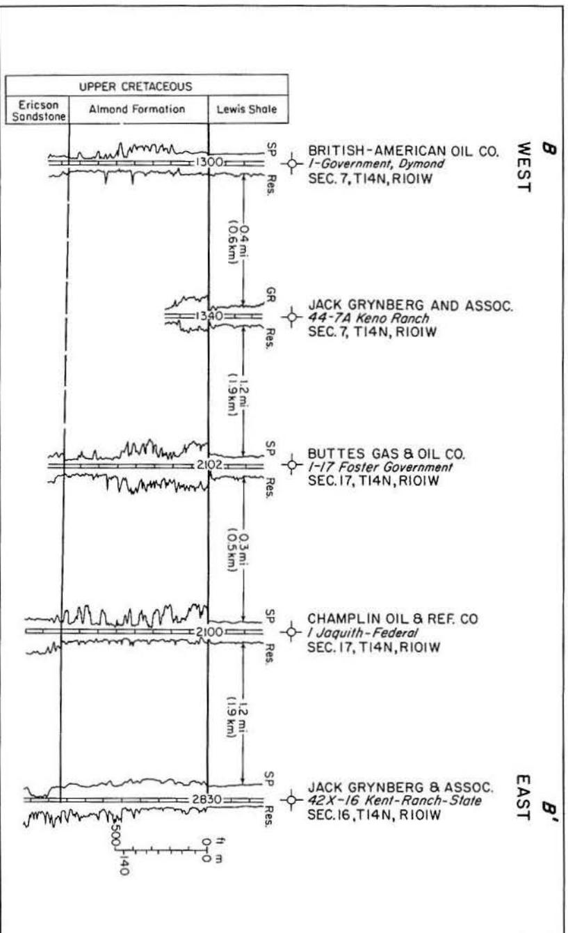
FIGURE 84. East-west stratigraphic cross section B-B' through the Almond Formation (undivided), Greater Green River Basin (after Tyler, 1980b).
