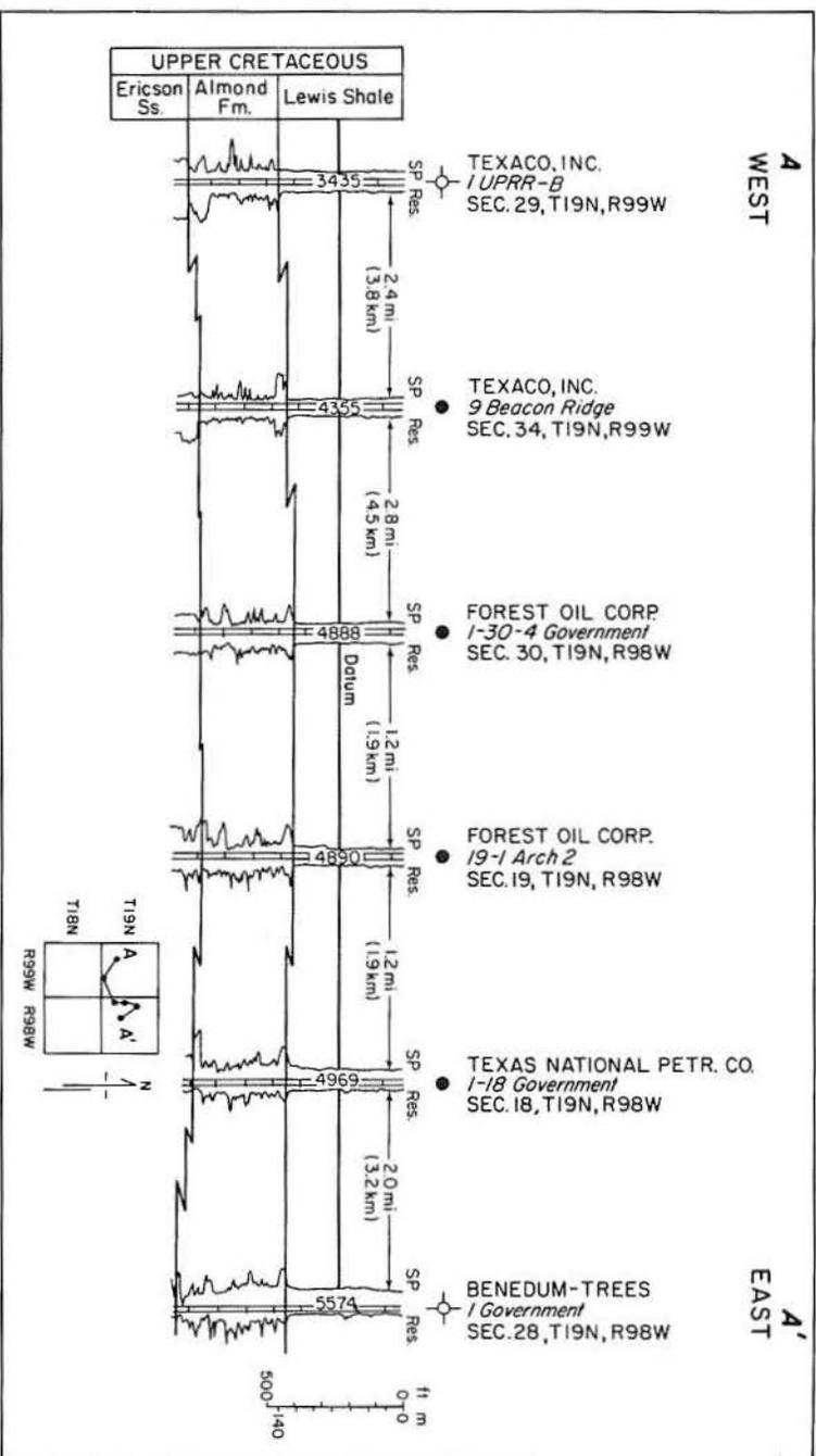
FIGURE 83. East-west stratigraphic cross section A-A' through the Almond Formation (undivided), Greater Green River Basin (after Tyler, 1978).
