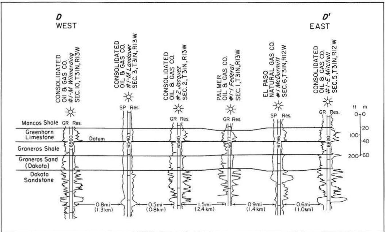
FIGURE 66. East-west stratigraphic cross section D-D' through the Dakota Sandstone and overlying strata, San Juan Basin (after New Mexico Oil Conservation Division, 1981b). Line of section shown in figure 62.
