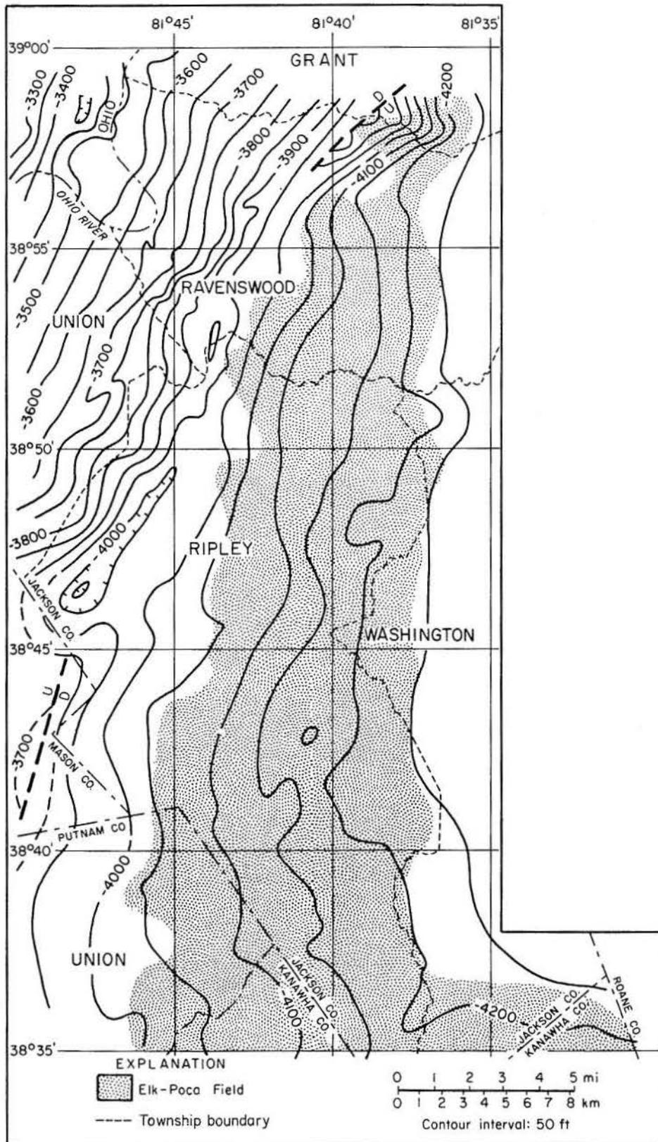
FIGURE 9. Structure contours on top of the Onondaga Limestone, Elk-Poca Field, North Sissonville area, West Virginia (from Diecchio, 1982b).
