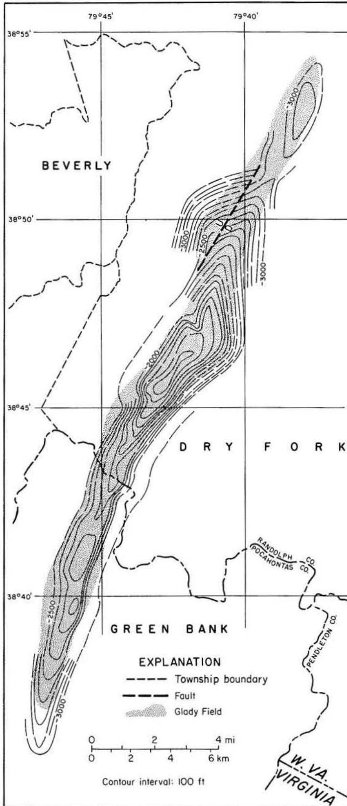
**FIGURE 12.** Structure contours on top of the Onondaga Limestone, Glady Field, West Virginia (from Diecchio, 1982b).
