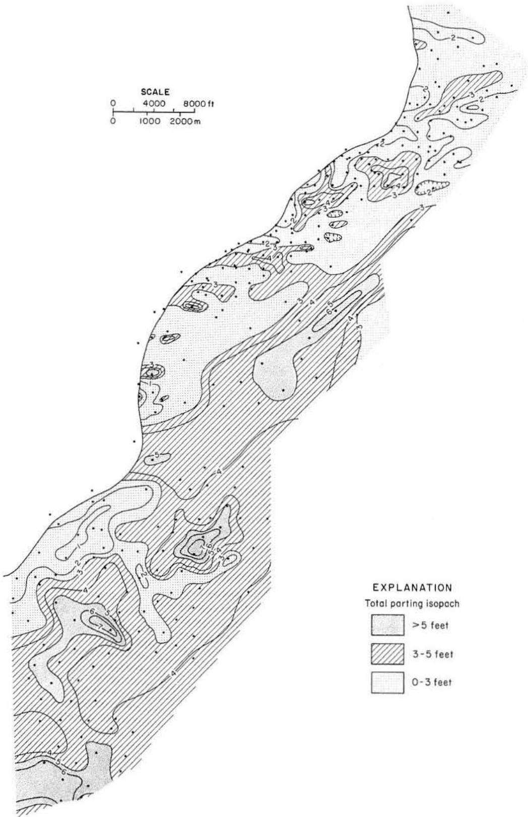
Figure 49. Isopach map of total parting thickness, seam no. 10, strandplain/lagoonal deposit, Jackson Group of South Texas.
