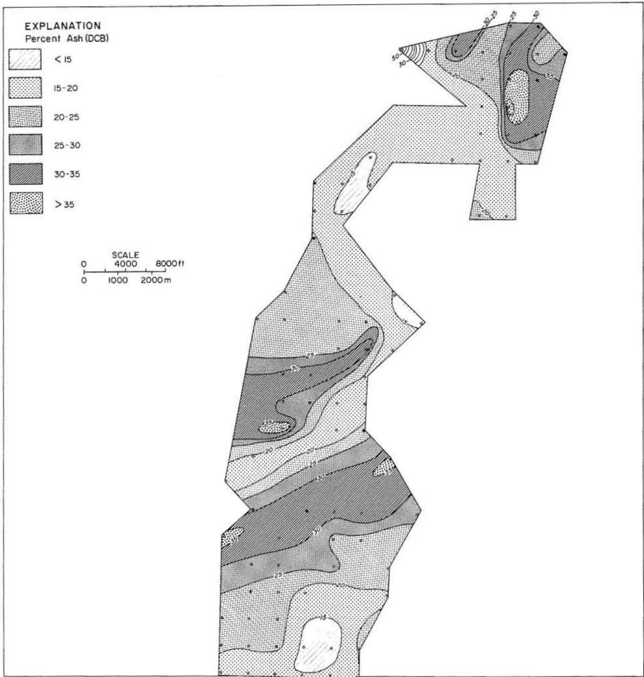
Figure 22. Isoline map of ash percent on a dry coal basis for seam no. 6, alluvial plain deposit, Wilcox Group of East Texas.
