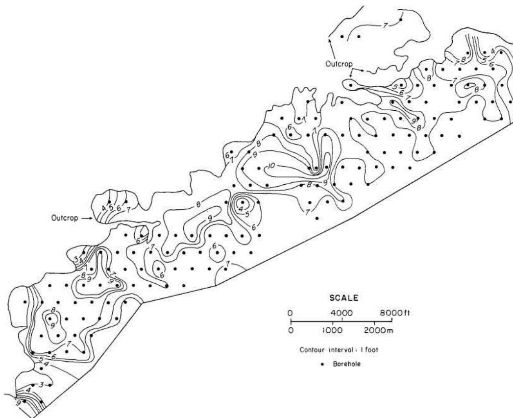
Figure 53. Isopach map of seam no. 3, 100 percent of available data, lower delta plain deposit, Jackson Group of southeast Texas.
