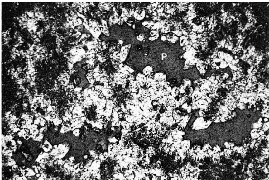
FIGURE 28. Network of fine-grained, dark calcite (C) and pyrite surrounding large pores (P) in the Oakwood anhydrite-calcite transition zone; depth is 907 ft (276.5 m). Photo width is 2.6 mm; plane light.
