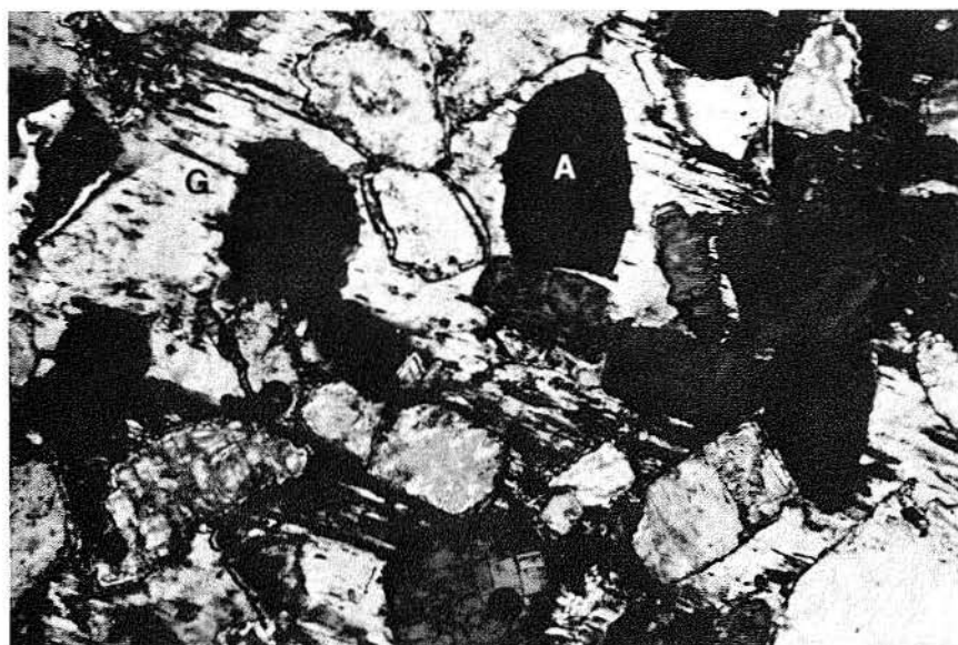
FIGURE 44. Poikilotopic gypsum cement (G) surrounding anhydrite crystals (A) in Rayburn's Dome cap rock; depth is 102 ft (31 m). Photo width is 2.0 mm; crossed nicols.
