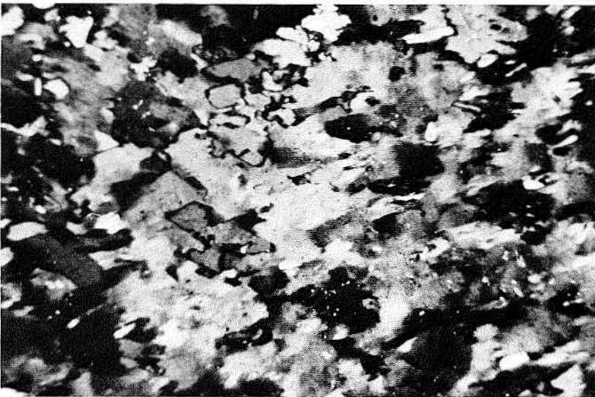
FIGURE 14. Highly strained, equigranular gypsum from Gyp Hill cap rock; depth is 15 ft (4.6 m). Black areas are all gypsum at extinction. Photo width is 2.6 mm; crossed nicols.
