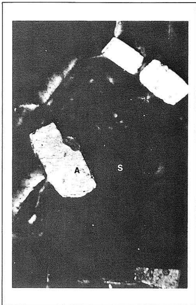
FIGURE 22. Anhydrite crystals (A) in Oakwood salt stock (S); depth is 1,163 ft (354.5 m). Photo width is 2.6 mm; crossed nicols.
