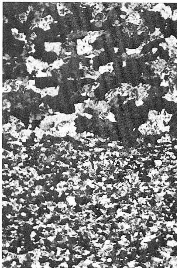
FIGURE 47. Contact between coarse- and fine-grained anhydrite layers in Vacherie Dome cap rock; depth is 588 ft (179.2 m). Photo width is 2.0 mm; crossed nicols.
