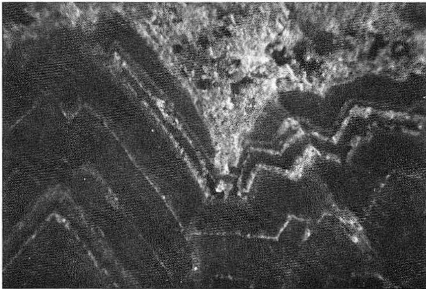
FIGURE 32. Coarsely crystalline, light calcite under cathodoluminescence, showing multiple growth zones. Sample from Oakwood cap rock at depth of 798 ft (243.2 m); photo width is 1.9 mm.
