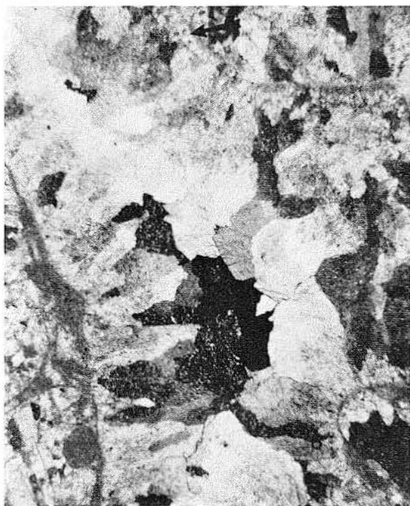
Figure 52. a and b. Strong evidence that at least some radial cement had an inversion origin includes the preservation of ghosts of original skeletal microstructure (arrows). c. Radial inversion of rudist shells, marked by the ghost of shell microstructure (arrow), is also common in the "cleaner" packstones of the shelf-margin facies. d. Micritization of skeletal walls (1), internal sediment (2), and neomorphism of allochems (3) occur in the shelf-margin wackestones.
