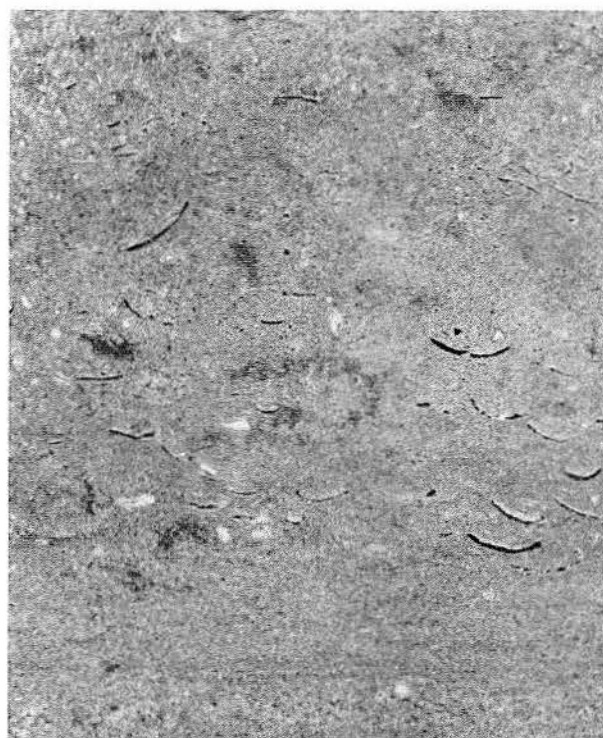
Figure 21. Laminated dolomite mudstone: a. Burrows disrupt oxidized laminae and possibly mud cracks (arrow) of this typical intertidal-supratidal dolomite mudstone; b. Nodular anhydrite in contorted organic-rich dolomite mud. Texture is characteristic of tidal-flat dolomite being replaced or displaced by anhydrite in the supratidal zone. Skeletal dolomite grainstone: c. Nearly 15 percent moldic porosity due to leached pellets. Original bedding completely destroyed by burrowing; d. Core slab very similar to (c) showing aligned and leached molluscan shells in pellet-rich matrix.
