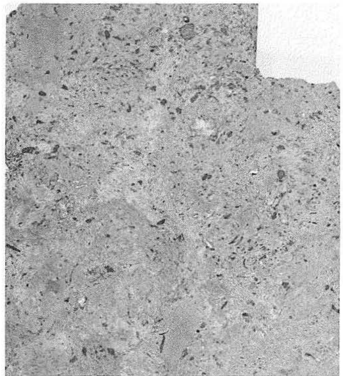
Figure 18. Burrowed dolomite mudstone: a. Very abundant burrows with oxidized rims suggest intertidal to supratidal deposition; b. Due to extensive burrowing, only minor original wispy lamination remains. Pellet-mollusk dolomite wackestone: c. Greater than 10 percent fossil moldic porosity exists, mainly between the large dark burrows; d. About 10 percent moldic porosity evenly distributed within and between burrowed areas.
