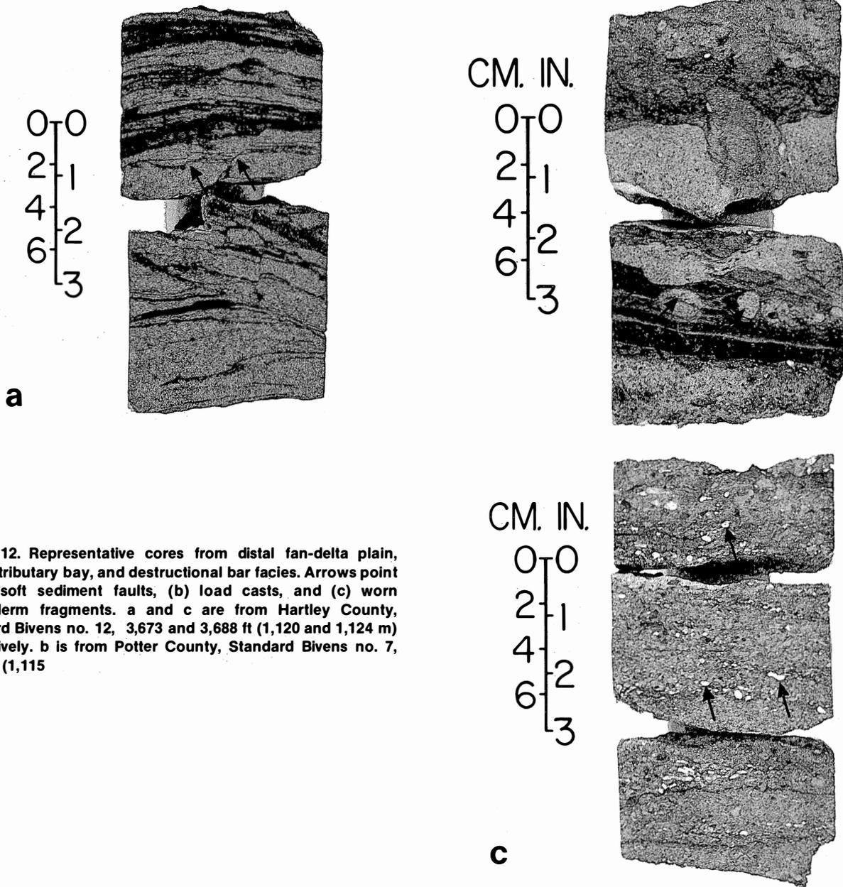
Figure 12. Representative cores from distal fan-delta plain, interdistributary bay, and destructional bar facies. Arrows point to (a) soft sediment faults, (b) load casts, and (c) worn echinoderm fragments. a and c are from Hartley County, Standard Bivens no. 12, 3,673 and 3,688 ft (1,120 and 1,124 m) respectively. b is from Potter County, Standard Bivens no. 7, 3,659 ft (1,115
