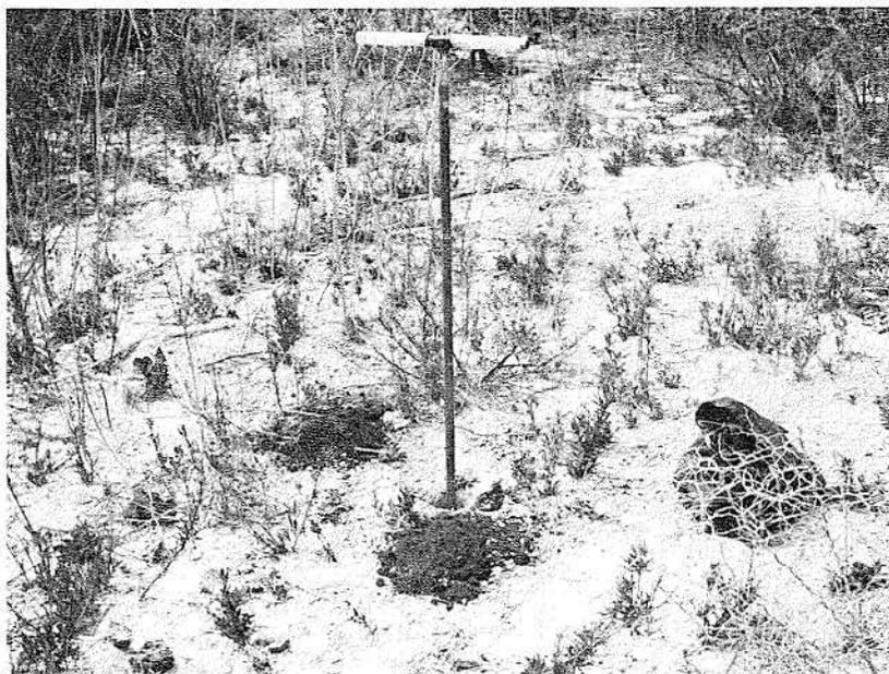
**Figure 14.** Sample location 18. Light-colored material is overburden eroded from spoil pile behind photographer. Dark material piled in front of sample hole is natural soil from beneath eroded overburden.
