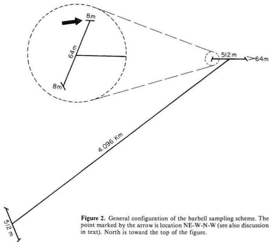
Figure 2. General configuration of the barbell sampling scheme. The point marked by the arrow is location NE-W-N-W (see also discussion in text). North is toward the top of the figure.
