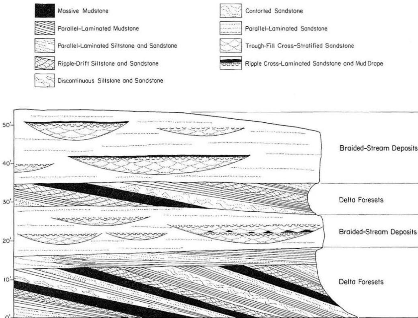
Figure 8. Schematic of fan-delta deposits in Oldham County, Texas (Boys Ranch 7.5-minute quadrangle), along right bank of Canadian River, west of U. S. Route 385 and south of Fort Worth and Denver Railroad. Shown here are (1) delta foresets consisting of (a) massive and parallel-laminated mudstone, (b) parallel-laminated siltstone and sandstone, (c) ripple-drift sandstone and siltstone, (d) discontinuous siltstone and sandstone (pull-aparts), and (e) contorted sandstone
