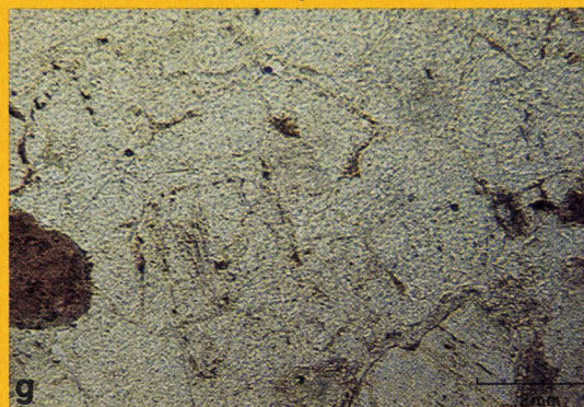
g. Massive quartz overgrowth welding has occluded the pore space. Frio Formation, Humble No. 1 Skrabanek (17,030 to 17,060 feet), Brazoria County, Texas.
