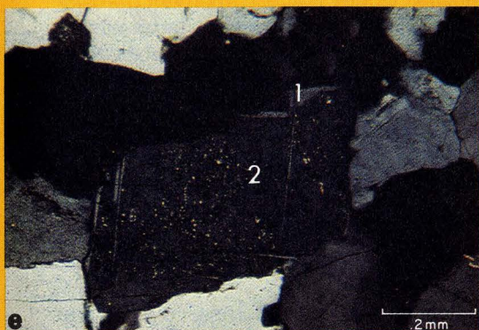
e. Authigenetic feldspar overgrowth (1) on plagioclase grain (2). Light specks in plagioclase grain are areas of calcite replacement. Crossed nicols. Frio Formation, Humble No. 1 Skrabanek (17,030 to 17,060 feet), Brazoria County, Texas.
