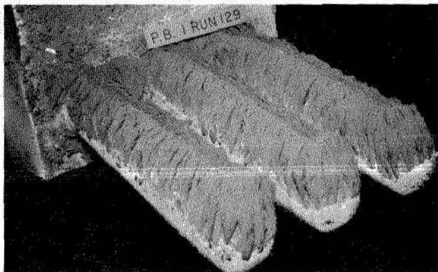
Figure 6. Comparison of probe deposits. (A) High-fouling lignite (weight, 315 g; ash, 10.3 percent dry basis; Na 2 O in ash, 6.5 percent). (B) Low-fouling lignite (weight, 35 g; ash 11.8 percent dry basis; Na 2 O in ash, 0.5 percent).
