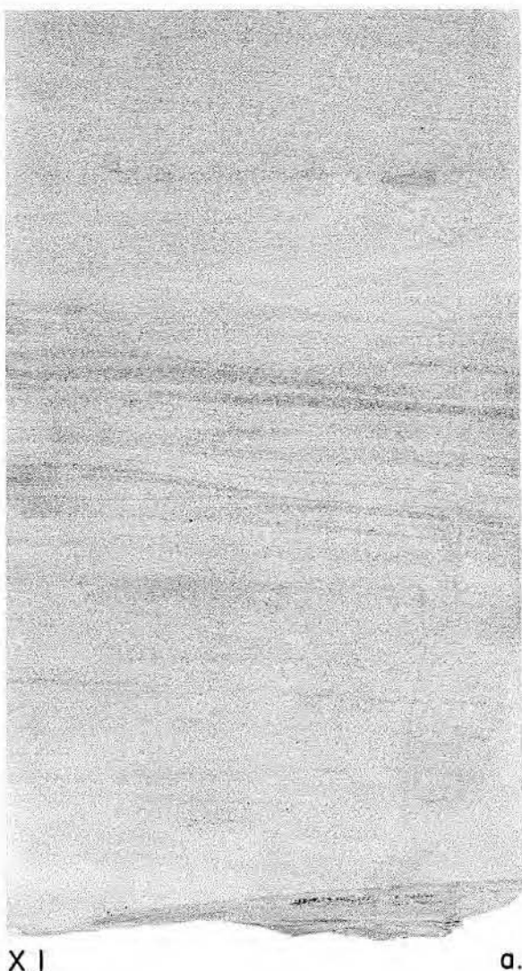
Figure 8. Laminated, cross-laminated, and rippled sandstone from the Hosston Formation. From the Magnolia No. 1 Mercer, Caldwell County, a-4,432 ft; b-4,411 ft.
