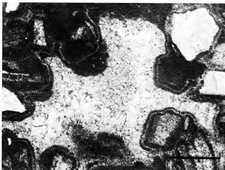
Figure 32. Photomicrograph showing a keystone vug at the top of a perireef grainstone (unit I). Fibrous isopachous cement (submarine phreatic?) is overlain by micritic meniscus cement (marine vadose?). The vug was filled later by equant sparry calcite (fresh-water phreatic). Bar scale is 250 microns.
