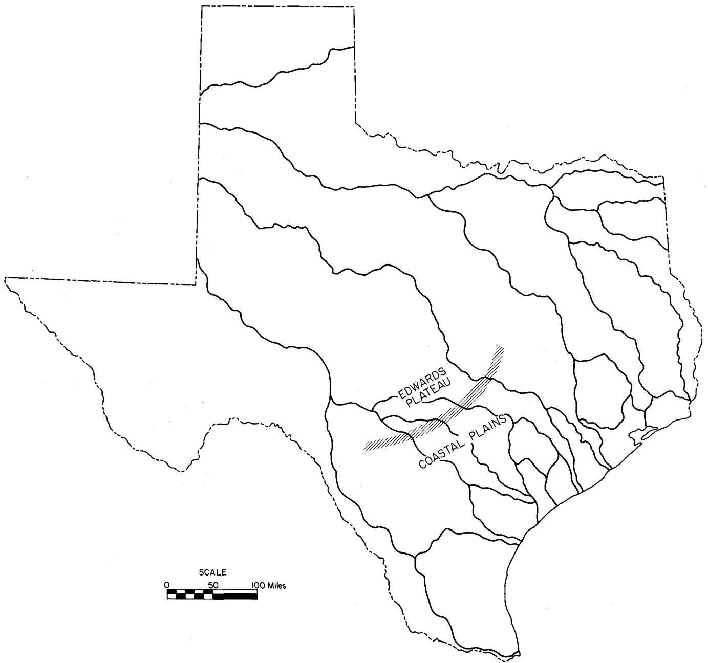
Figure 2. The Edwards Plateau-Coastal Plains boundary heads several drainage basins. Line pattern locates the Balcones fault zone and related escarpment.
