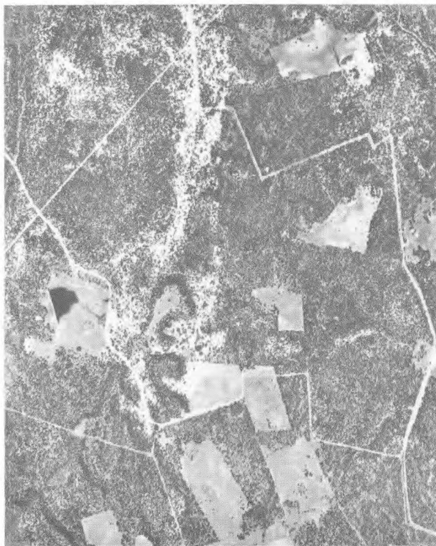
Figure 7. Environmental geologic units: HRIC, high-relief iron-cemented uplands; SH, sand hills. On an aerial photograph and topographic map of a portion of the Thomas Springs quadrangle. (U.S.G.S. topographic map, Thomas Springs Quad., Tx.; aerial photograph reproduced with permission of Tobin Surveys, Inc.)
