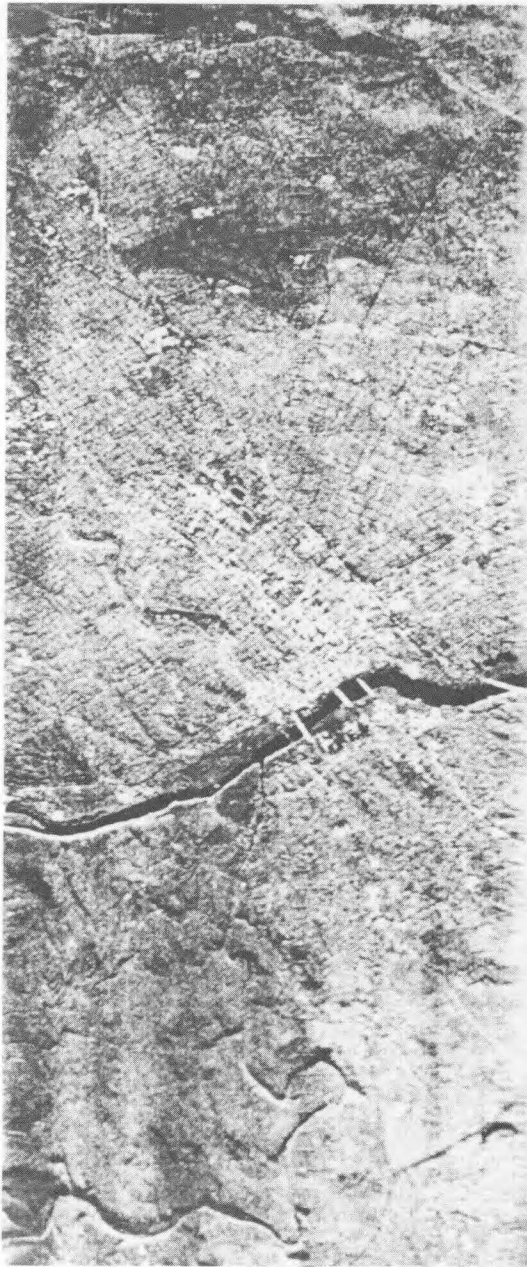
Figure 3. Radar imagery of the heart of Austin, Texas. Individual metropolitan features can be easily identified. The high-return areas in the center of the image are due to the large buildings of downtown Austin, the Capitol complex, and The University of Texas, which reflect large amounts of the propagated radar energy back to the aircraft.
