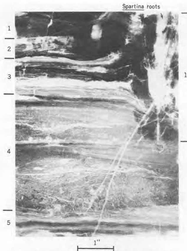
FIG. 34. Radiograph of low marsh sediment. Sample taken from Spartina alterniflora marsh lying along the distal fan in the low between the middle and eastern lobes.
