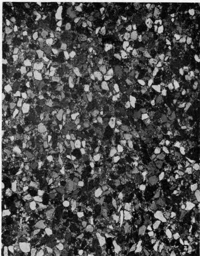
Calcareous, fine-grained quartz sandstone (under cross nicols). From approximately 5 feet above the base of the Paluxy Sandstone near Pinyan Creek, southeast of Bertram, Burnet County, Texas. Sample P-2, \times 36 .
