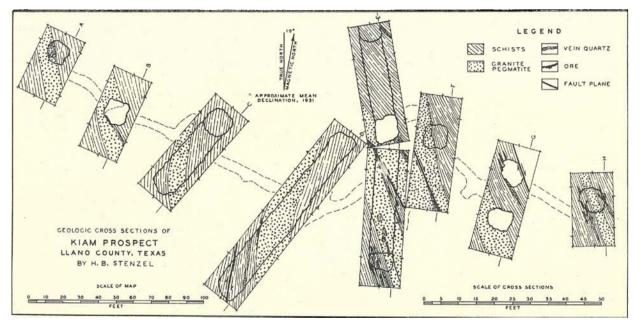
Fig. 137. Geologic cross sections of the underground workings of the Kiam prospect, Llano County. Texas.
