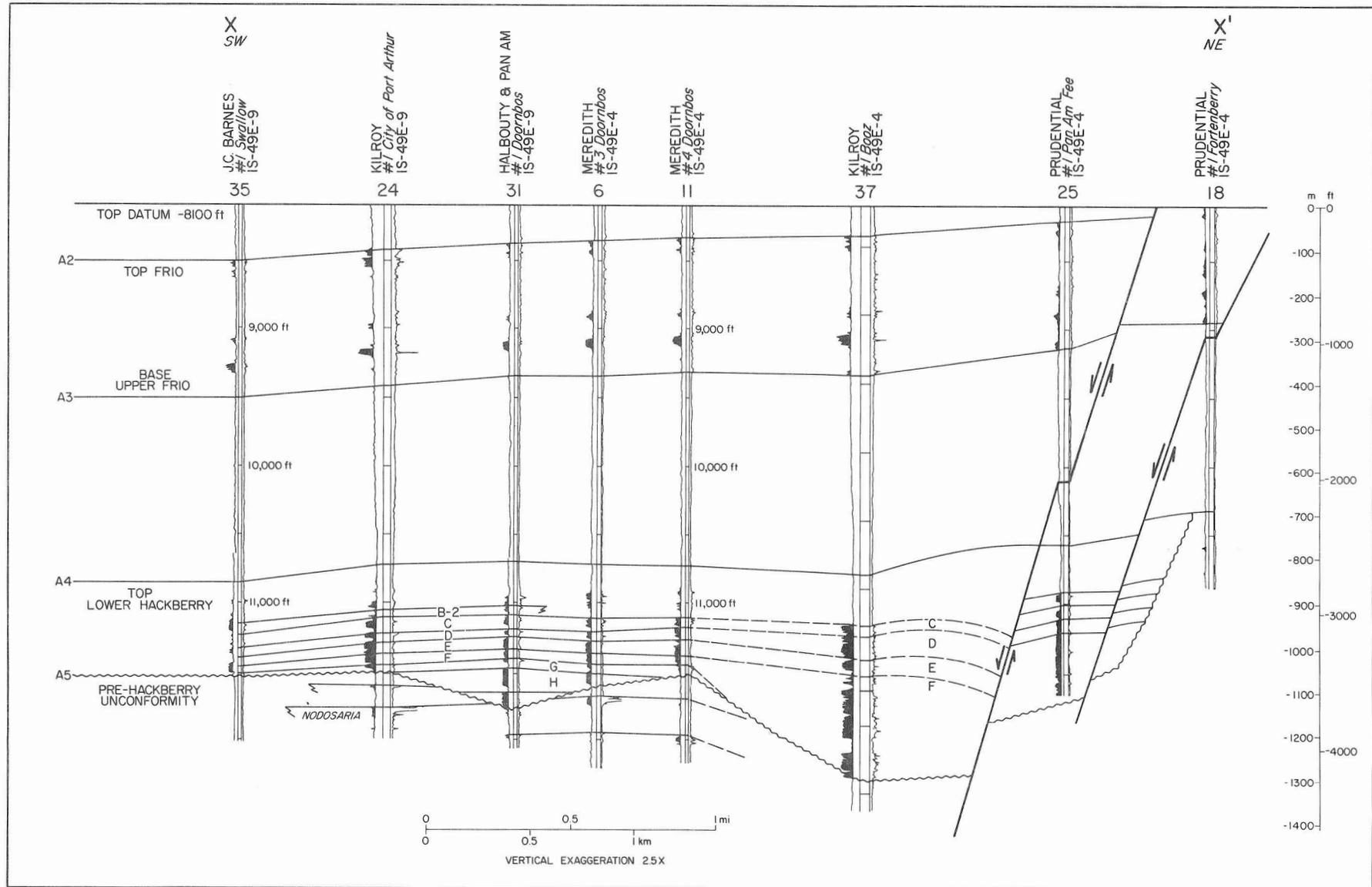
Figure 11. Structural section X-X' across Port Arthur field showing named sand units within the lower Hackberry, the relation of the main field to the large channel and growth fault, and the log characteristics of the sands. Line of section is shown in figure 10.
