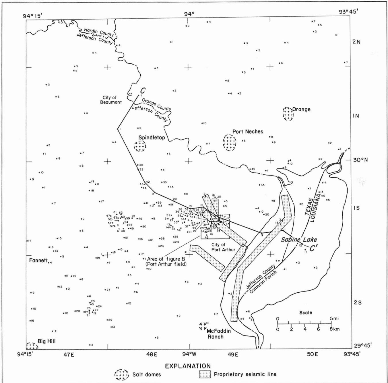
Figure 4. Location map of the Port Arthur area showing wells used for correlation and general locations of seismic lines and line of cross section C-C' (fig. 5).
