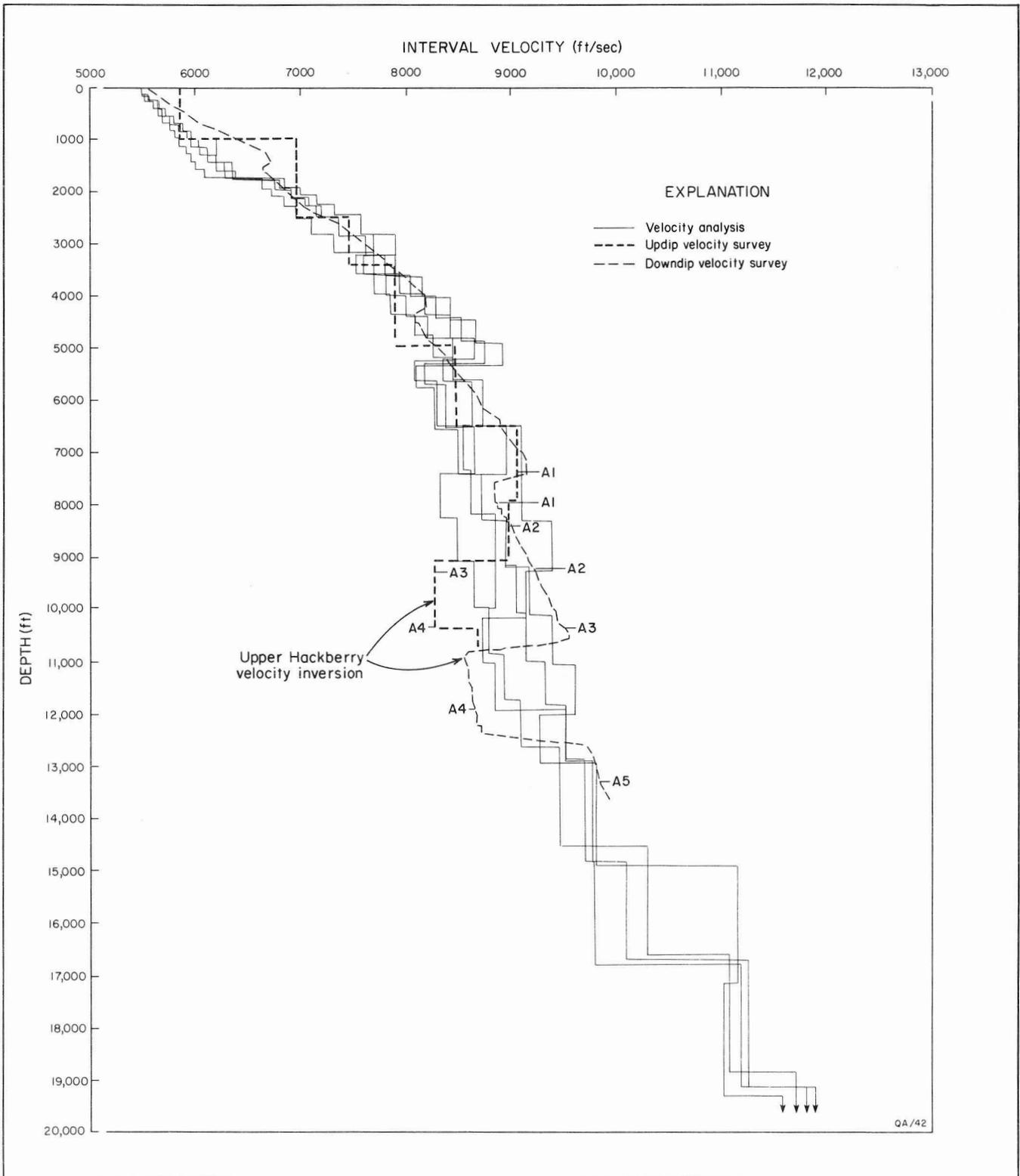
Figure 6. Interval velocity versus depth for two velocity surveys and velocity analyses from seismic data. Stratigraphic horizons are shown for the two well surveys. The surveys show a velocity inversion between A3 and A4.
