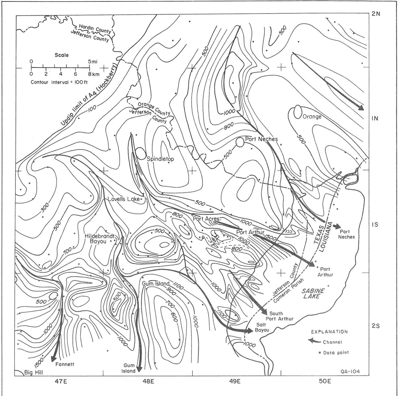
Figure 7. Isopach map of the A4 through A5 interval (lower Hackberry), Port Arthur area. Several large channel axes are woven together by minor channels that surround isolated high areas on the pre-Hackberry unconformity.
