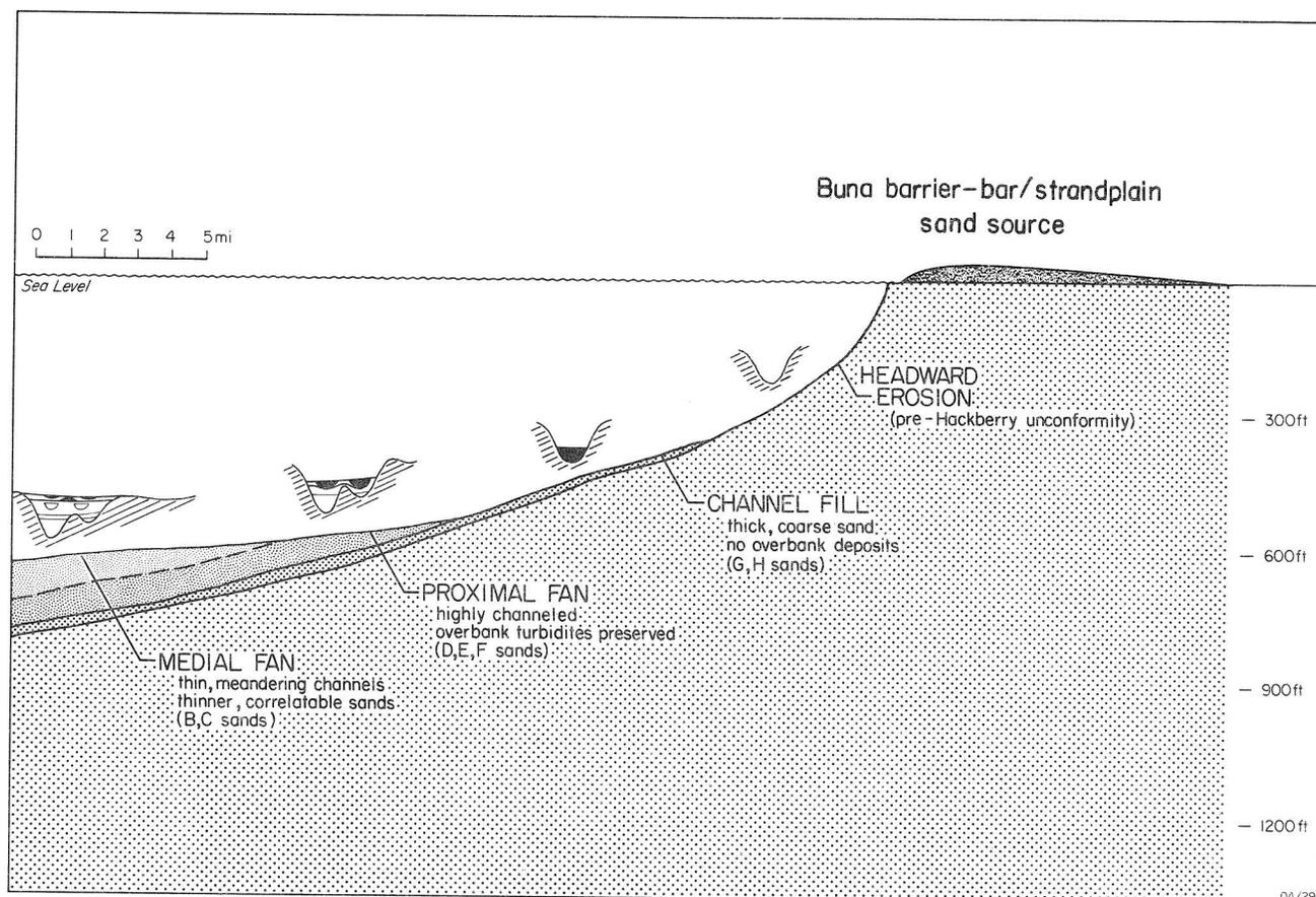
Figure 14. Onlapping submarine fan depositional model of lower Hackberry sand in the Port Arthur field. Channel sandstones are shown in black on the channel cross sections.
