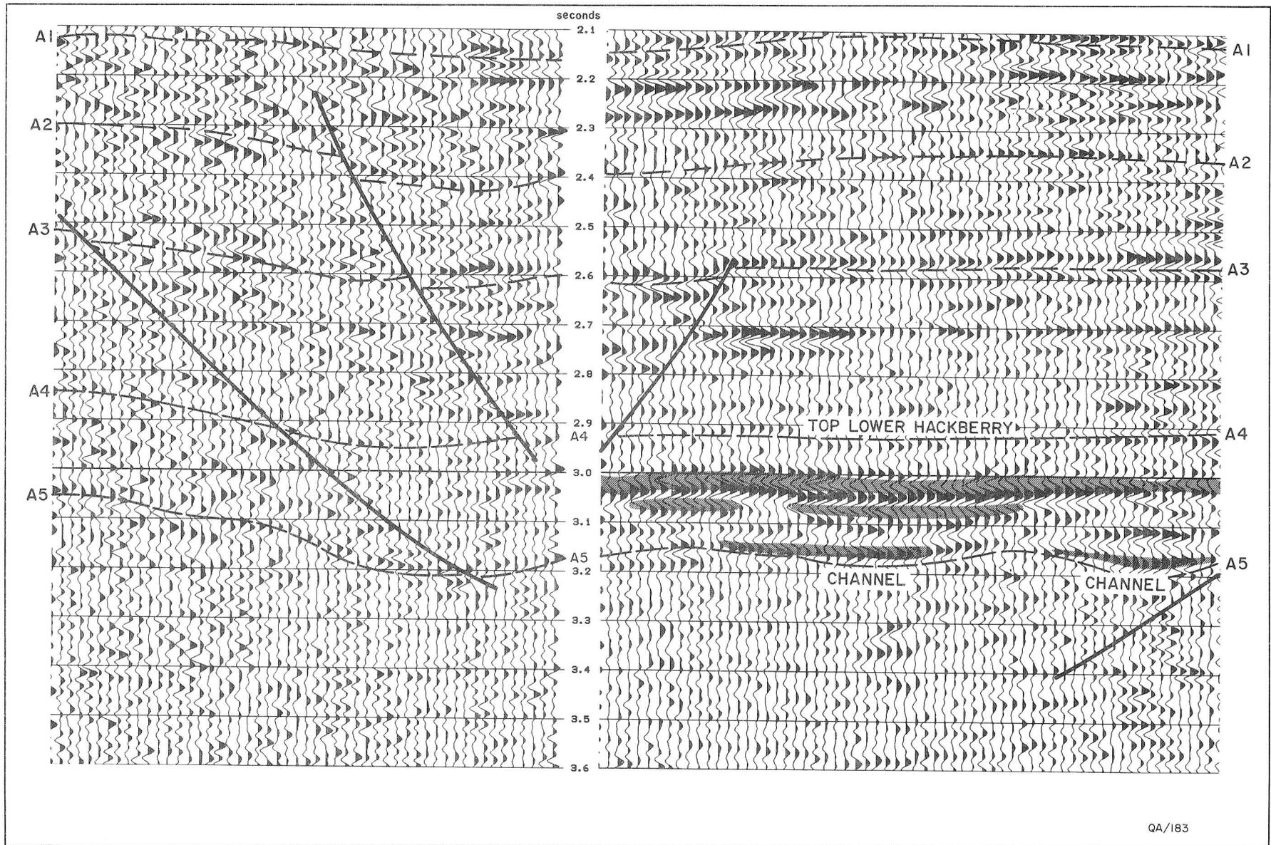
Figure 15. Seismic reflection character of the Hackberry in wavelet-processed, migrated dip (left) and strike (right) lines. Note the extremely poor reflector quality in the dip-oriented data and the submarine channels shown in the strike-oriented data.
