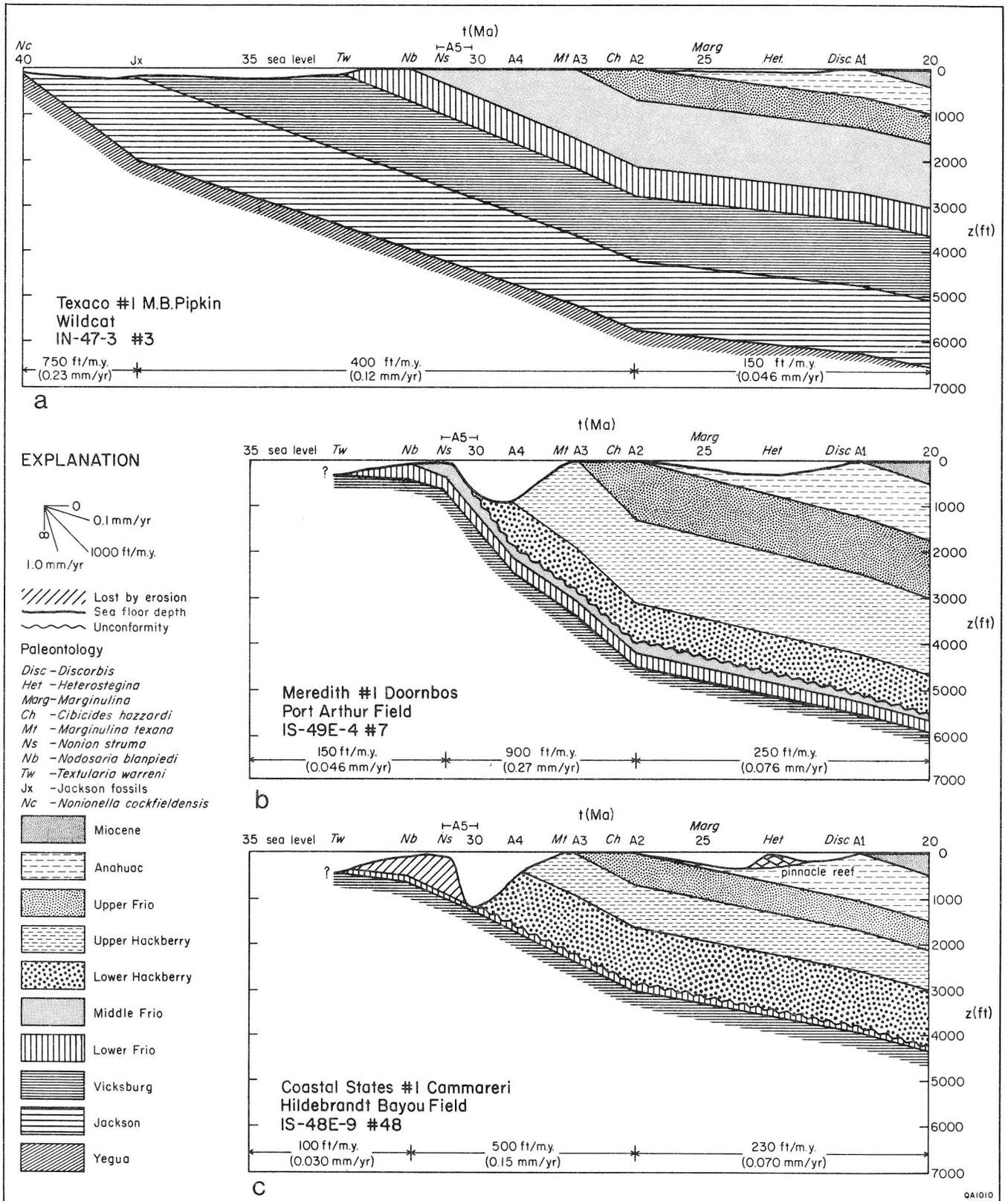
Figure 19. Time-depth curves for three wells in Jefferson County showing reconstructed water depths and subsidence and sedimentation history for (a) a well updip of the embayment, (b) a well in Port Arthur field (interchannel), and (c) a well in the Gum Island channel. Location of wells is shown in figure 4.
