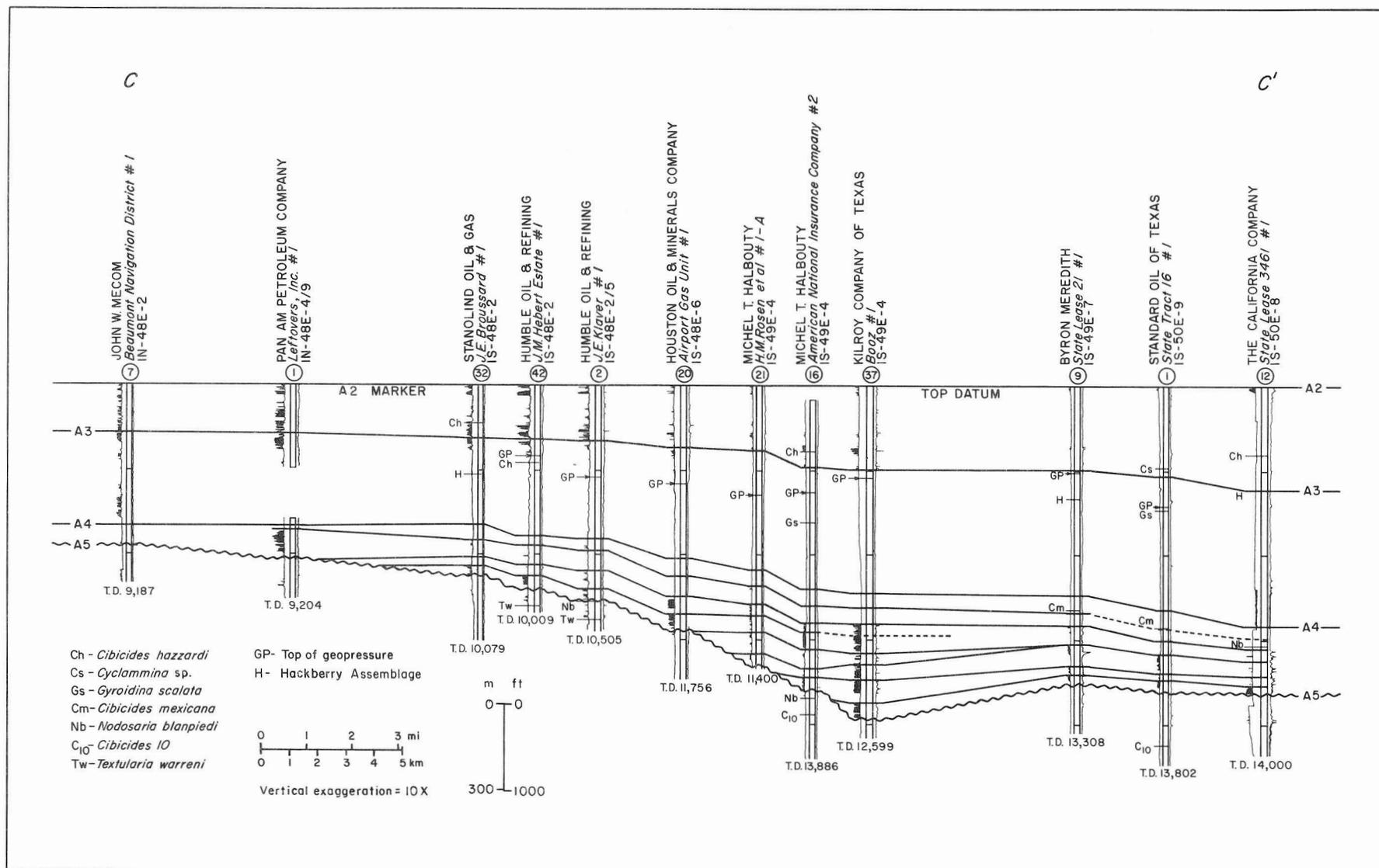
Figure 5. Stratigraphic section C-C' of Hackberry and upper Frio sands along the major channel near Port Arthur field. A possible sand-package correlation is shown, suggesting progressive onlap of the deep-water sandstones against the pre-Hackberry unconformity. Several of the wells used are marginal to the main channel. Also note the seaward progradation of the upper Frio sandstones. Line of section is shown in figure 4.
