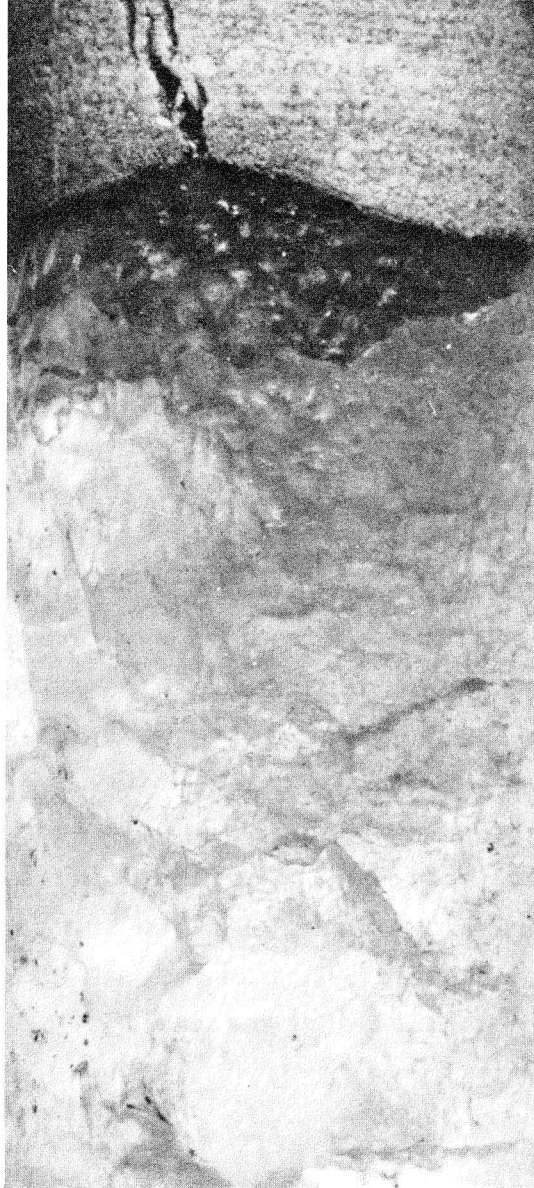
Figure 54. Photograph of tight contact between salt and overlying cap rock (from Dix and Jackson, 1982). Core is 10 cm (4 inches) wide.
