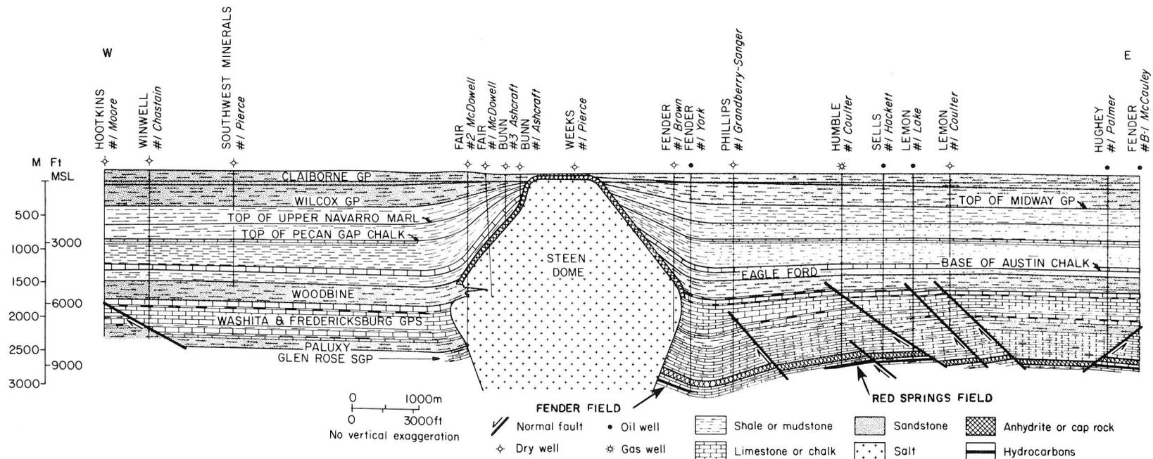
Figure 12. West-east structure section across Steen Dome, Smith County, Texas; a turtle-structure anticline is east of the dome. Dome location shown in figure 1. Data for the Ashcraft wells were supplied by J. R. Bunn.
