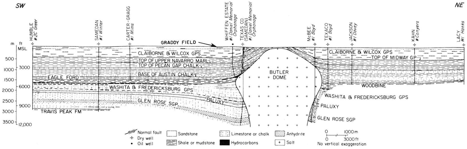
Figure 14. Southwest-northeast structure section across Butler Dome, Freestone County, Texas. Dome location shown in figure 1.
