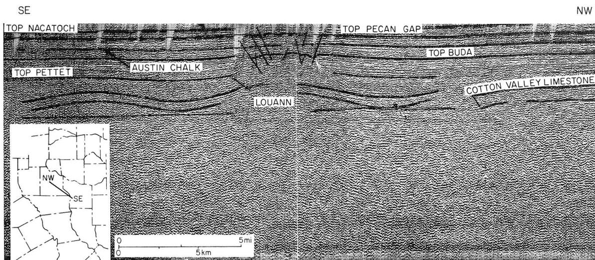
Figure 5. Southeast-northwest seismic section across the Van Dome area. Unmigrated seismic section courtesy of Teledyne Exploration Company. The crestal anticline and associated faults trap hydrocarbons over the deep salt pillow. Dome location shown in figure 1.
