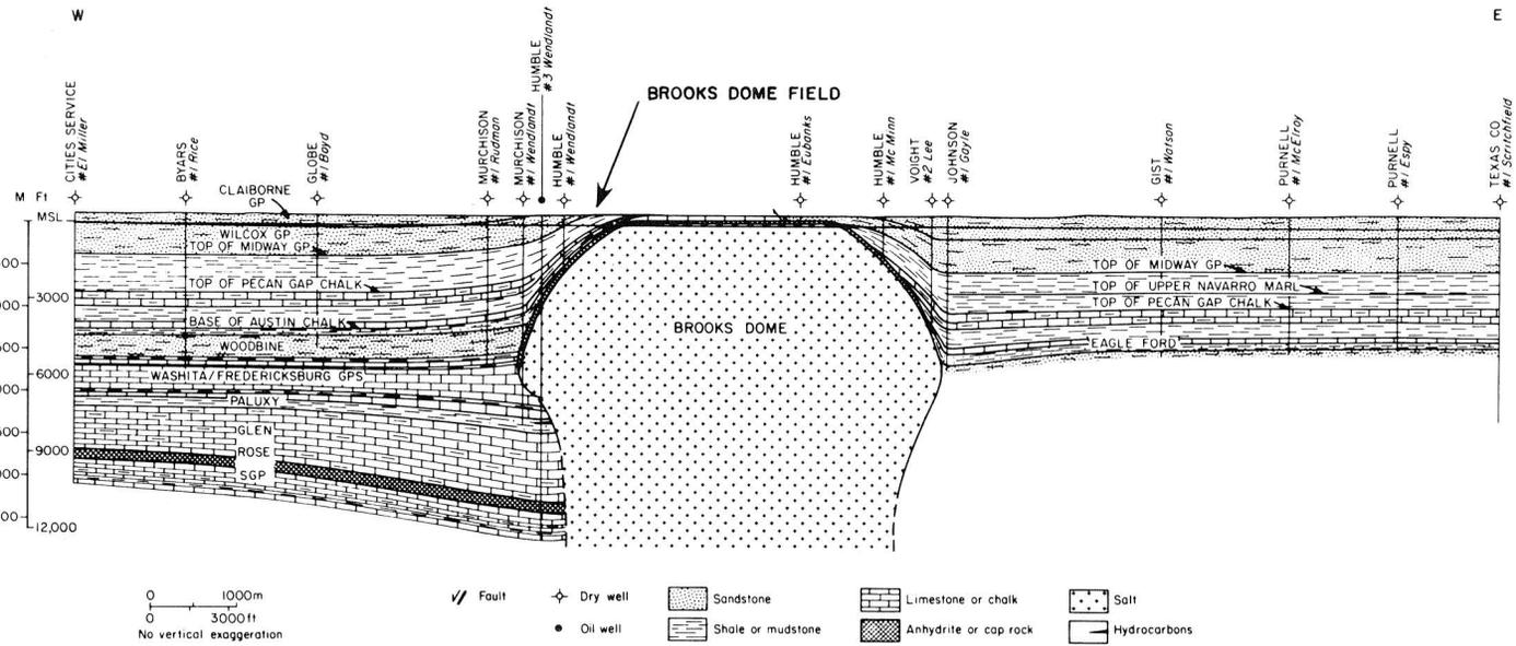
Figure 17. West-east structure section across Brooks Dome, Smith County, Texas. Dome location shown in figure 1.
