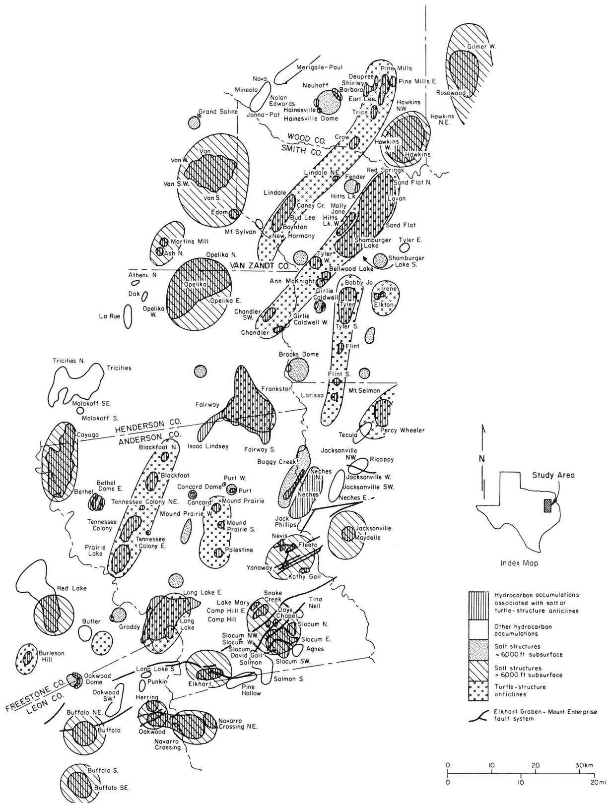
Figure 8. Shallow salt domes (salt structures <6,000 ft deep), salt-cored anticlines (salt structures >6,000 ft deep), turtle-structure anticlines, and hydrocarbon fields of the central East Texas Basin.
