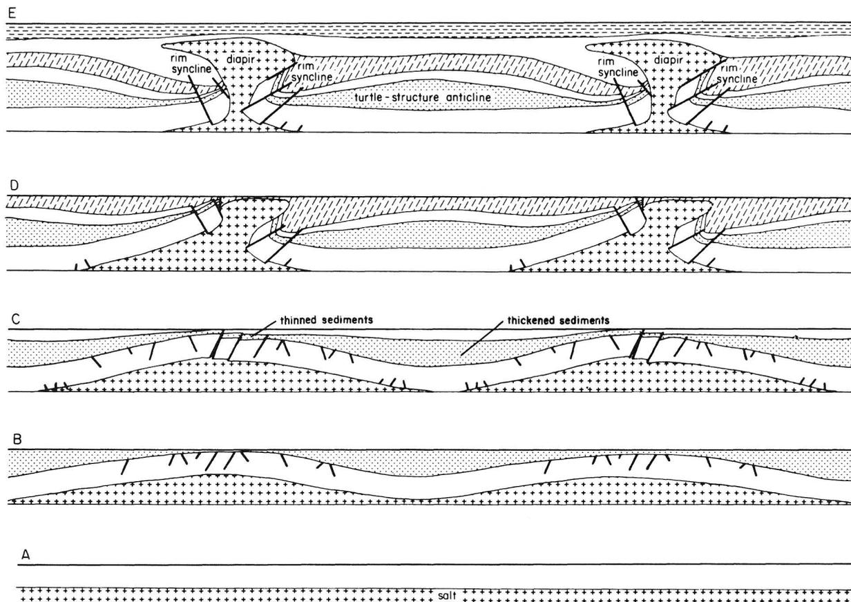
Figure 7. Model of evolution of salt domes and turtle-structure anticlines A through E (modified from Trusheim, 1960). A. Initial configuration. B, C. Salt pillow stage with distant rim syncline. D, E. Salt diapir stage. Rim syncline is adjacent to dome. Turtle-structure anticline is fully developed.
