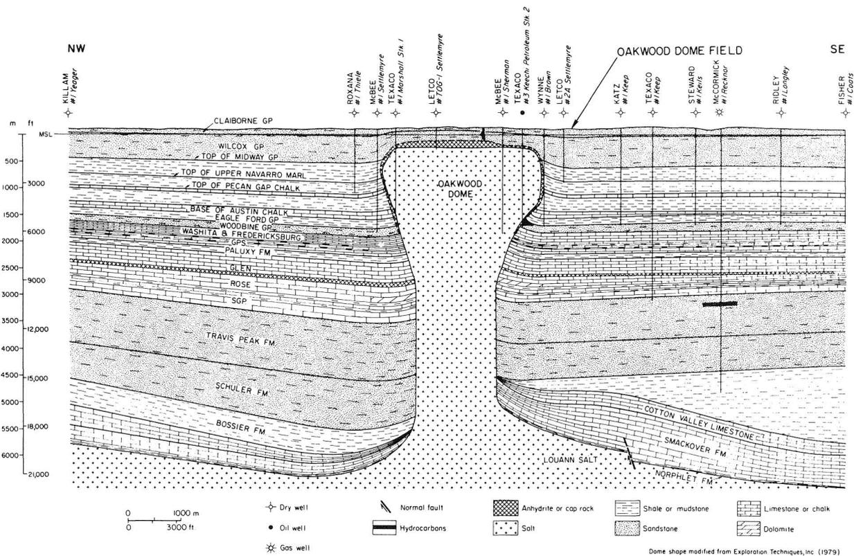
Figure 15. Northwest-southeast structure section across Oakwood Dome, Freestone and Leon Counties, Texas. Geology based partially on seismic profile. Dome location shown in figure 1.
