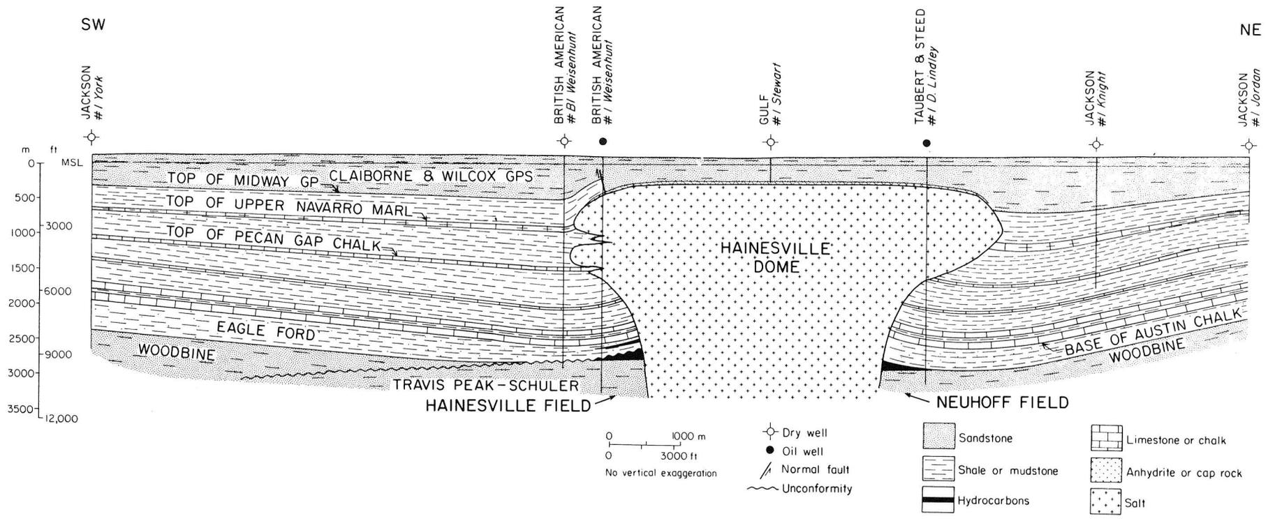
Figure 16. Southwest-northeast structure section across Hainesville Dome, Wood County, Texas. Dome location shown in figure 1.
