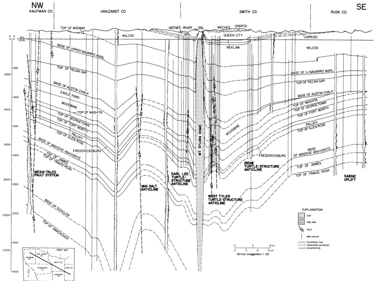
Figure 2. Northwest-southeast dip section across the East Texas Basin. Movement of salt deformed Jurassic, Cretaceous, and Tertiary strata and created diapirs, salt-cored anticlines, and turtle-structure anticlines. Salt diapirs such as Mount Sylvan Dome developed along the central axis of the basin.
