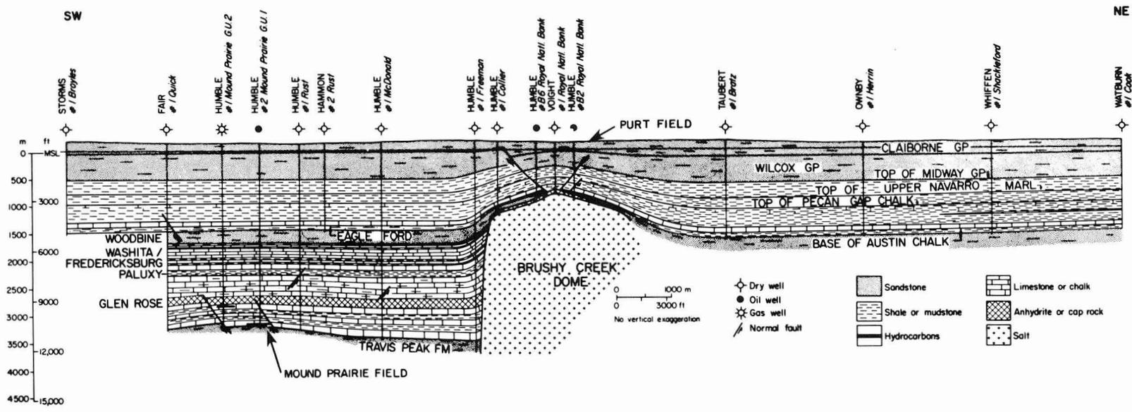
Figure 13. Southwest-northeast structure section across Brushy Creek Dome, Anderson County, Texas. Dome location shown in figure 1.
