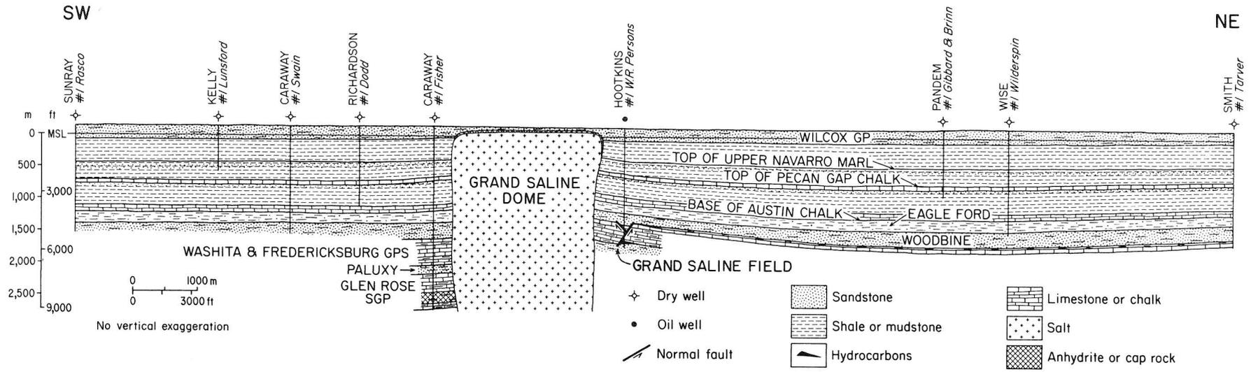
Figure 18. Southwest-northeast structure section across Grand Saline Dome, Van Zandt County, Texas. Dome location shown in figure 1.
