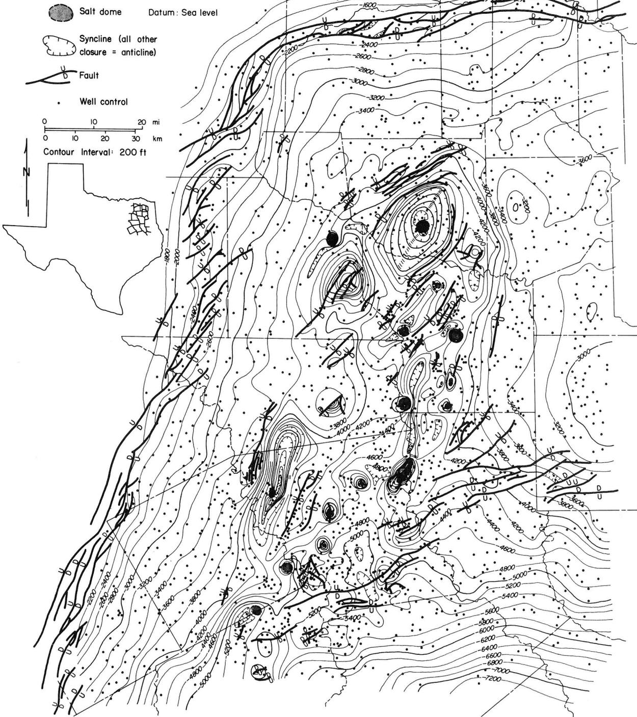
Figure 3. Structure map of the base of the Austin Chalk in the East Texas Basin showing deformation of strata caused by salt movement. Datum is sea level. Faults modified from Geomap Company (1980).
