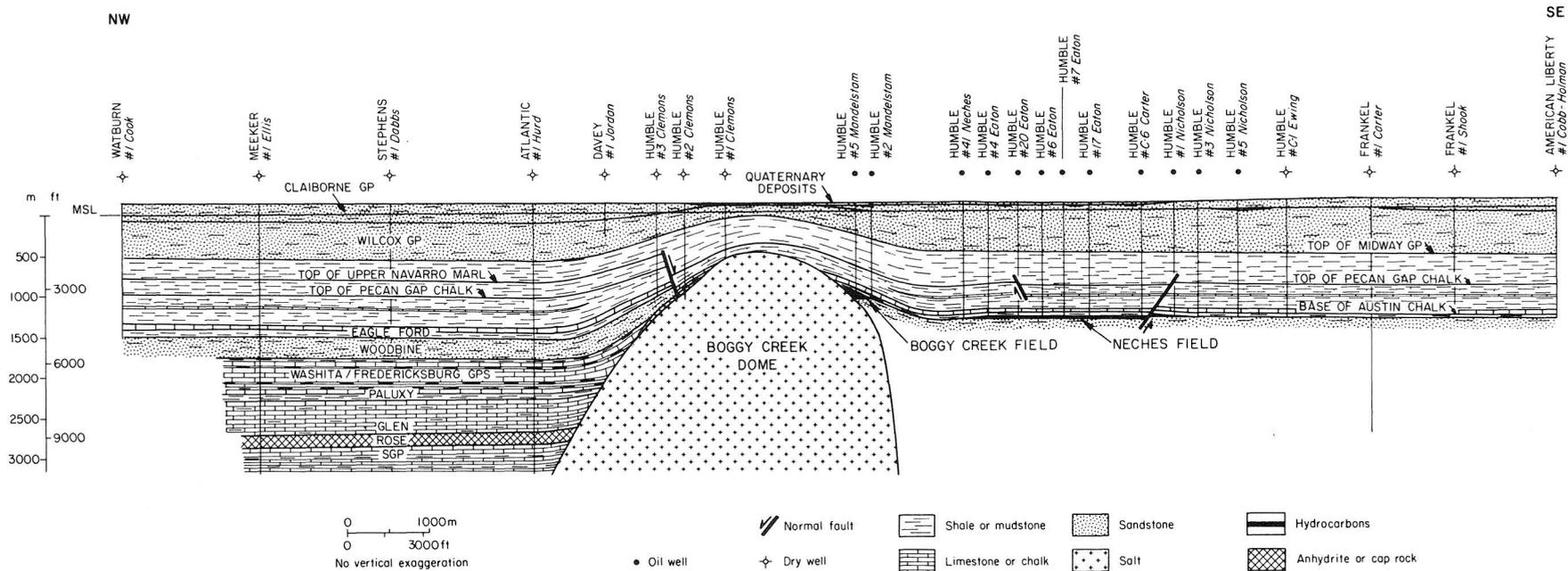
Figure 10. Northwest-southeast structure section across Bogy Creek Dome, Anderson and Cherokee Counties, Texas. The Bogy Creek field produces from strata on the flank of the dome; the Neches field produces from the turtle-structure anticline southeast of the dome. Locations shown in figure 1.
