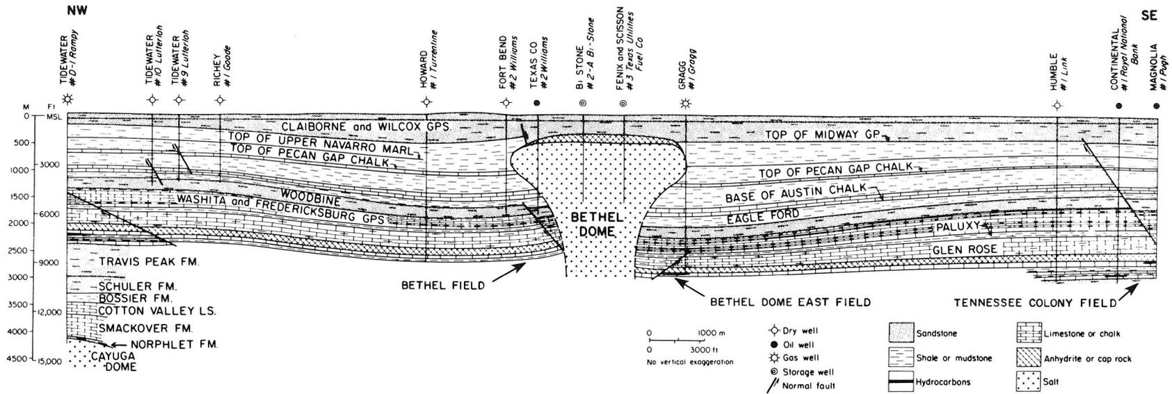
Figure 11. Northwest-southeast structure section across Bethel Dome, Anderson County, Texas, with a turtle-structure anticline southeast of the dome. Dome location shown in figure 1.
