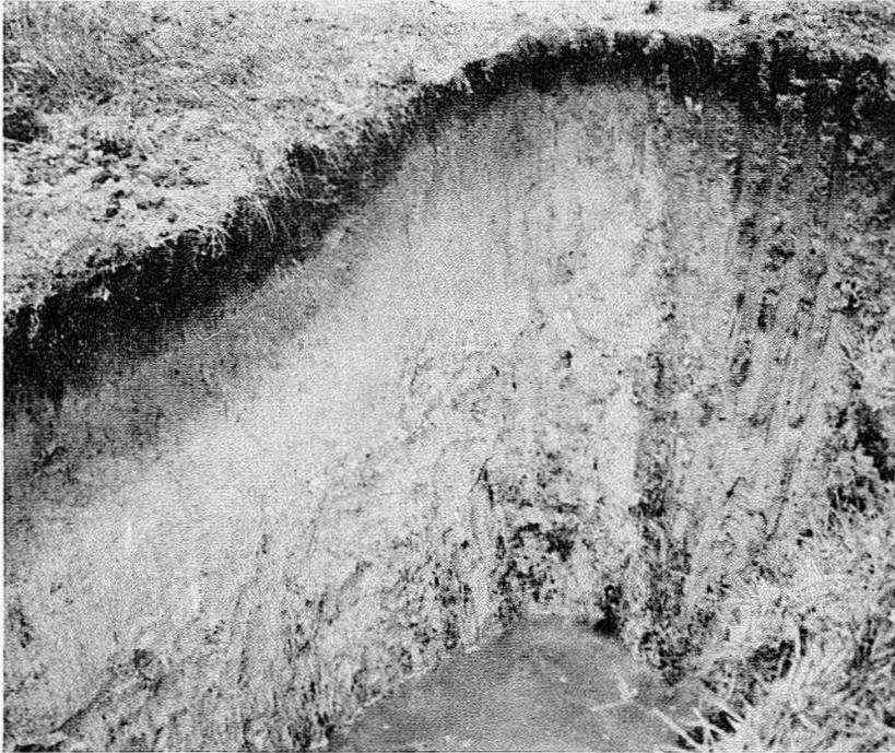
Figure 11a. Trench across Library fault, Ellington Air Force Base. Note thickening of soil profile on downthrown side of fault. No fault plane surface evident.
