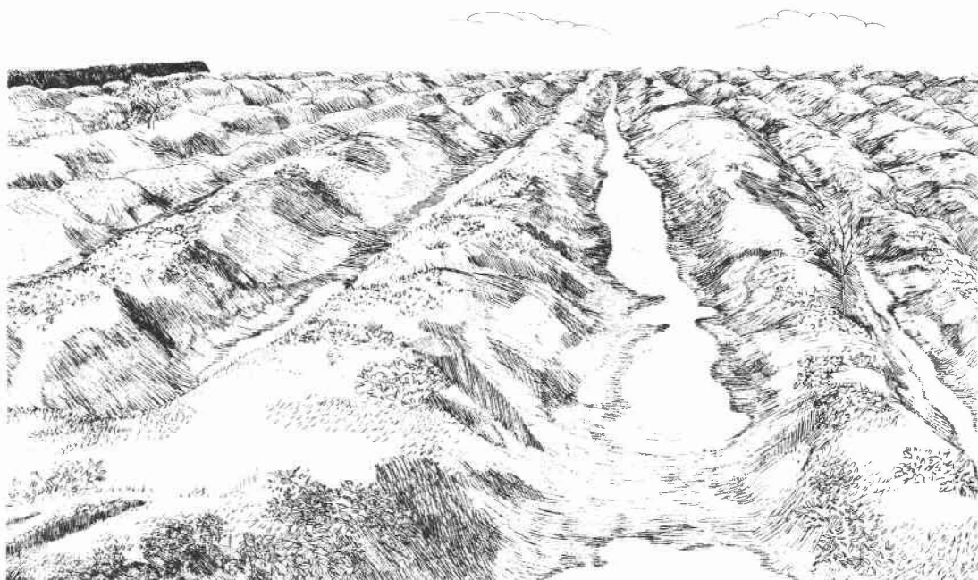
Figure 2. Appearance of land mined for sand and gravel by the area stripping method.
