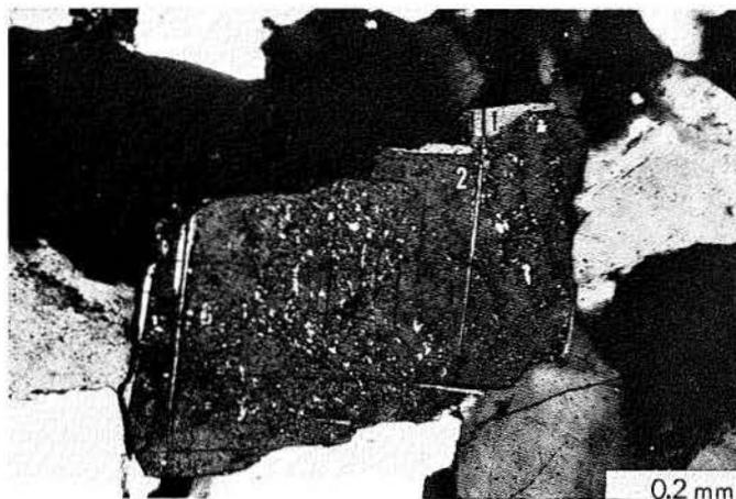
**FIGURE 12.** Authigenetic feldspar overgrowth (1) on plagioclase grain (2). Light specks in plagioclase grain are areas of calcite replacement. Crossed nicols. Frio Formation, Humble No. 1 Skrabanek (17,030-60 feet), Brazoria County, Texas.
