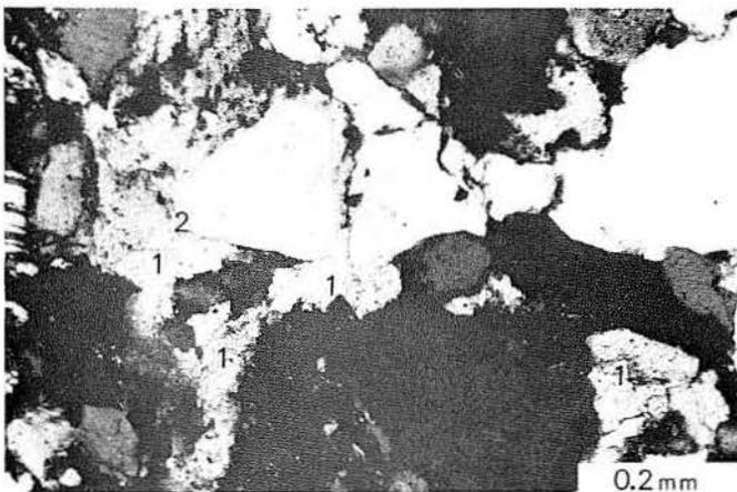
**FIGURE 15.** Sparry calcite cement (1) following quartz overgrowths (2). Pore space is totally filled. Crossed nicols. Frio Formation Humble No. 1 Skrabanek (16,130-60 feet), Brazoria County, Texas.
