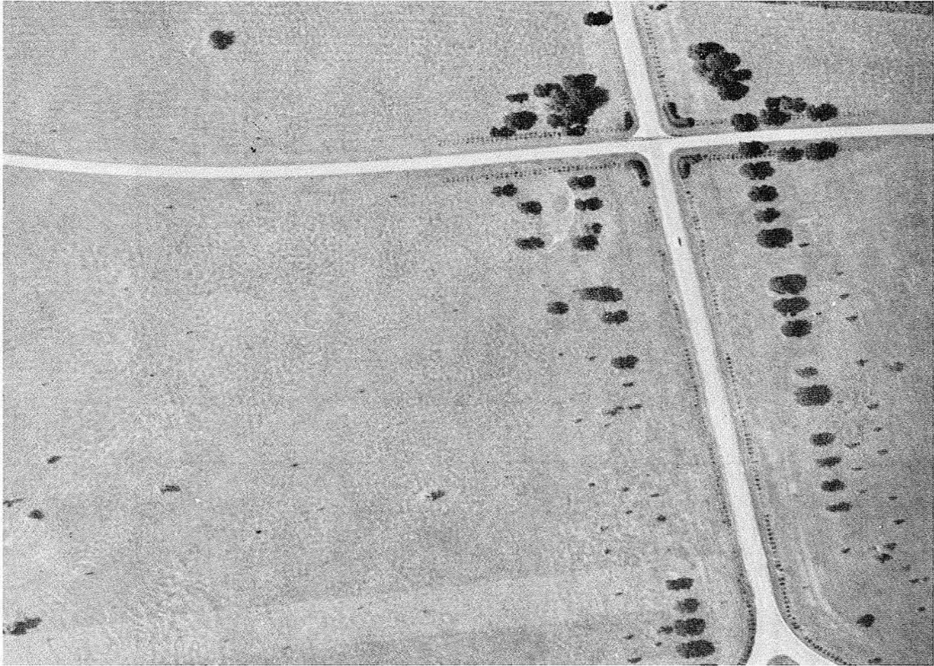
Figure 3B. Low altitude oblique aerial photograph of the surface of the Beaumont Clay near Houston, Texas. The near-level surface is covered with an irregular network of microridges (light toned) and microdepressions (dark toned). Roadways are approximately 35 feet wide
