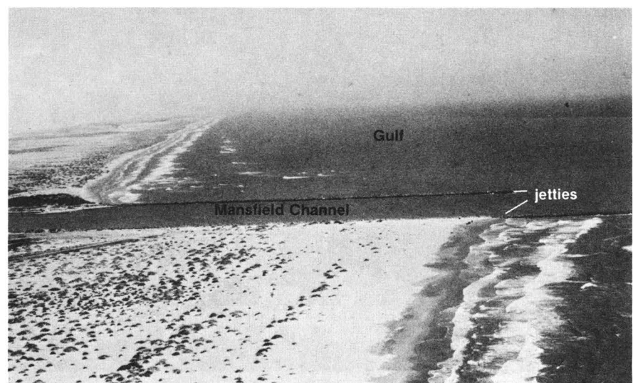
Figure 24. Jetties at Mansfield Channel. View is toward northwest. Note that sediments have accumulated on the south side of the jetties, which indicates that net longshore drift is northward at this location. Erosion has occurred on the north, or downcurrent, side of the jetties. The jetties are located in grid C-21 on plate I.
