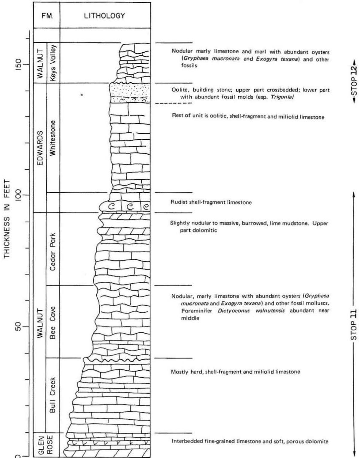
FIG. 24. Stratigraphic section at STOPS 11 and 12. STOP 11 is road cut in Travis County on north side of Ranch Road 1431, 2 miles west of Williamson County line. STOP 12 is inactive quarry of Texas Quarries, Inc., on south side of Ranch Road 1431 at Travis-Williamson County line (modified from Moore, 1964).
