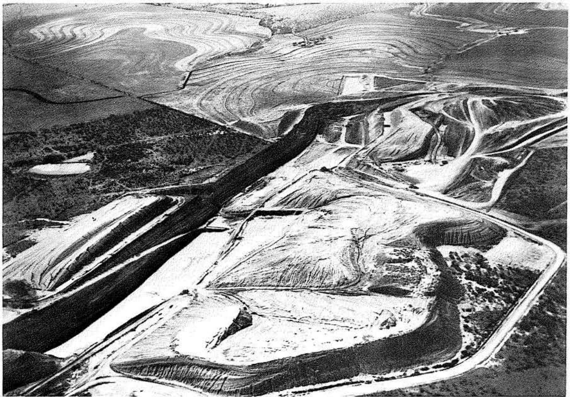
Figure 12 Oblique aerial photograph showing Susquehanna-Western's Butler-Weddington mine. The ore is at a depth of 100 to 130 feet along the bottom of the long trench. Some of the overburden is piled in high mounds at the sides of the trench; some has been back-filled as mining has progressed. (Photograph by Mitchell Photography, Kenedy, Texas.)
