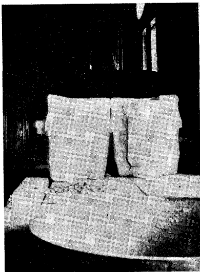
FIG. 11. PLASTER MOLD FOR CASTING, AT POTTERY PLANT AT FORT WORTH
