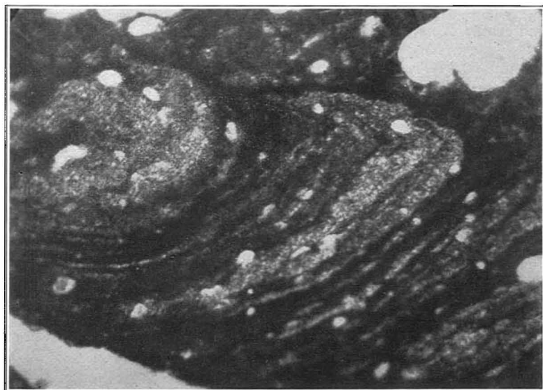
Fig. 2. Photomicrograph of fused shale showing flow structure. \times 26 .
