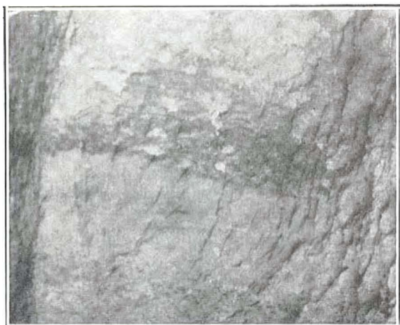
a. Entrance to the northeast drift at 16 in sketch map. Showing contact between the dark, gypsiferous material, and the brown, earthy material above. There is a great deal of kaolin-like sulphur in the dark material. A picked sample from the opposite side of this drift contained 54.4 per cent of free sulphur Michigan Sulphur and Oil Co.
