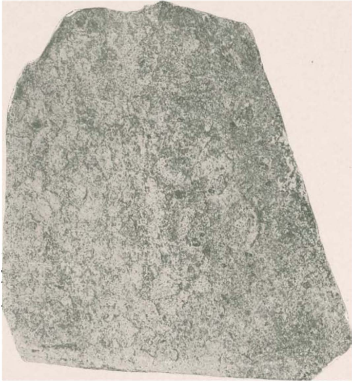
Plate 4....Photograph of a piece of chlorite rock said to have come from well no. 164, at somewhere from 727 to 917 feet below the surface. The photograph shows the polished surface of the rock. Natural size.
