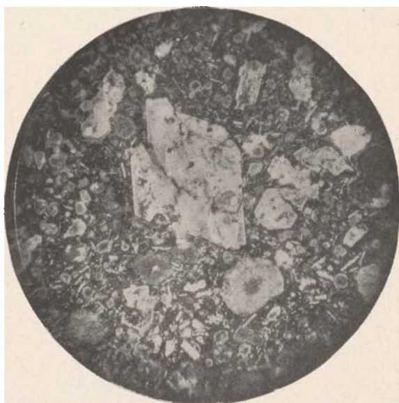
Plate 5....B...Micro-photograph of a thin section of altered igneous rock taken from well No. 73, showing the structure of the original basalt. Plane polarized light. Magnified about 40 diameters. Photograph by W. H. Tomlinson.
