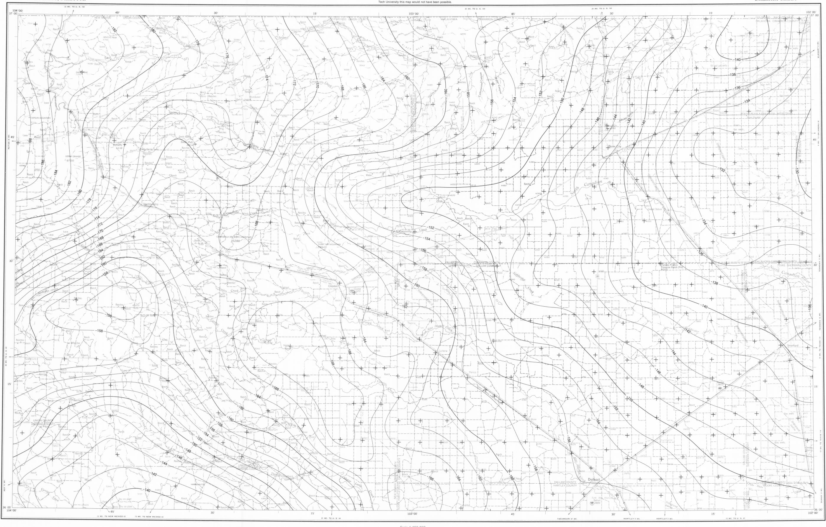
Prepared by the Army Map Service (BEGN), Corps of Engineers, U.S. Army, Washington, D.C. Compiled in 1955 by photogrammetric methods. Horizontal and vertical control by USGS, USC & GS, USCE and U.S. Soil Conservation Service. Aerial photography taken 1954. Photography field annotated 1954. Minor corrections by U.S. Geological Survey 1962.
