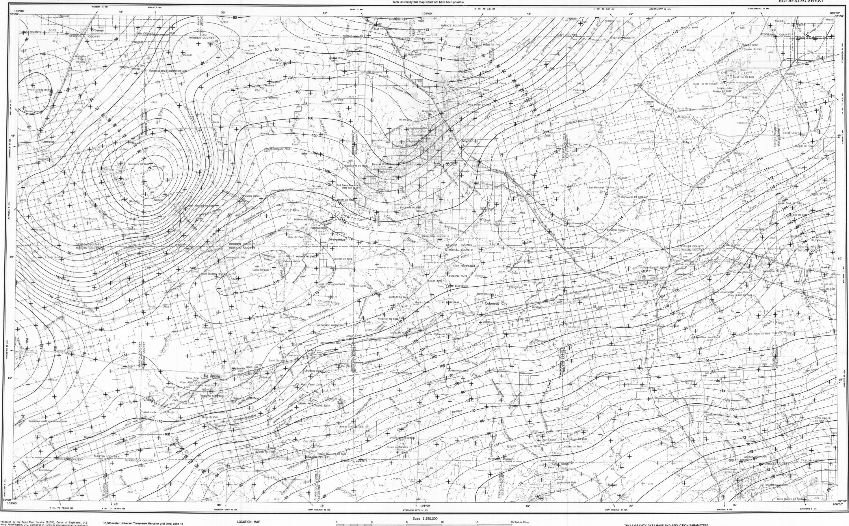
Prepared by the Army Map Service (AJSX), Corps of Engineers, U.S. Army, Washington, D.C. Compiled in 1954 by photogrammetric methods. Horizontal and vertical control by USGS. Aerial photography 1954. Photography field annotated 1954.
