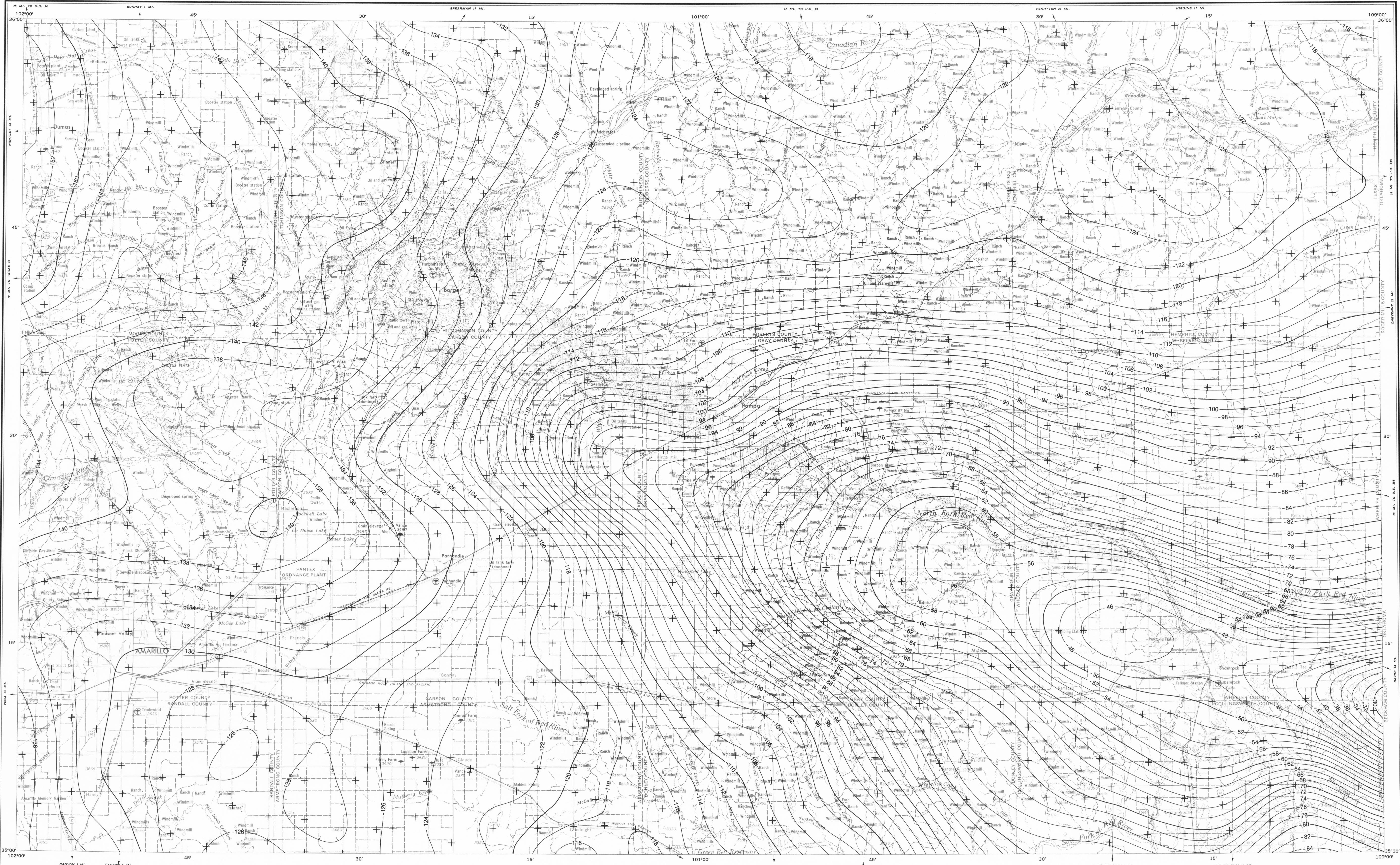
Prepared by the Army Map Service (BESX), Corps of Engineers, U.S. Army, Washington, D.C. Compiled in 1955 by photogrammetric methods and from Texas, 1:24,000, USGS, 1953. Planimetric detail revised by photo-planimetric methods. Horizontal and vertical control by USGS & GSC. Photography field annotated 1954.
