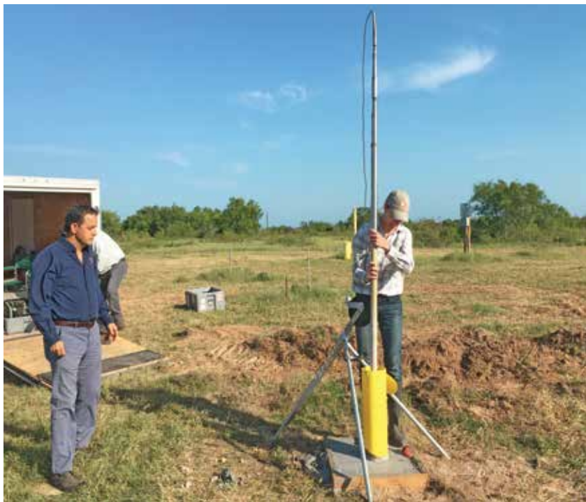
Mohsen Ahmadian looks on as Lucie Costard adjusts an EM induction logging tool.
