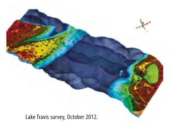
information? Just as in the system the Bureau has purchased, the downward-focusing sensors are installed on aircraft, and these combine many technologies to measure distances and other properties of reflected surface materials. A modern airborne lidar system installed on an aircraft will consist of a laser-beam
