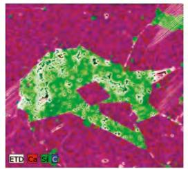
Bitumen sample imaged in EDS map mode.
