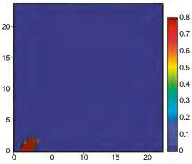
Quarter crack on an x-y plane. Note failed region around crack, which is due to applied pressure on the crack surface. Blue region represents intact material, whereas red region designates failed zone, which is due to locally developed tensile stress. This failed zone suggests development of microcracks around cracks that result from hydraulic fracturing.
