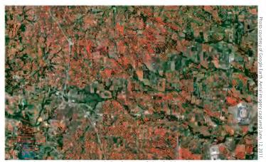
From geology to technology and the future of the field—drainage areas (in red) of existing wells, showing space left for future drilling.
