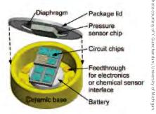
Millimeter<sup>3</sup>-scale integrated prototype system being developed by the AEC, integrating time-stamped chemical, pressure, temperature metadata in a high-pressure, high-temperature-capable package in collaboration with researchers at the University of Michigan, Cal Tech, Rice, and Boston University. Multichip module (top) and ceramic packaging (bottom).
