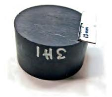
Barnett shale core plug used for gas-permeability measurement.
