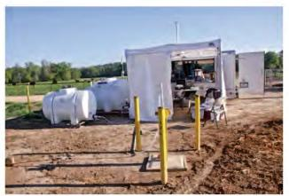
Push-pull test conducted at Cranfield site for assessing potential impacts of  $CO_2$  leakage from geological  $CO_2$  sequestration on groundwater drinking resources.
