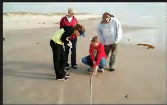
Port Aransas High School students are measuring how far their float (notice the orange on the beach) traveled in 50 seconds. This distance will help them calculate longshore current speed.
