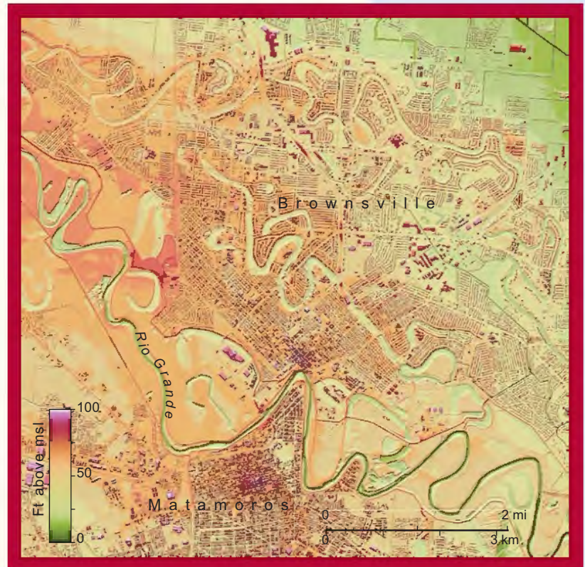
Digital elevation model of Brownsville, Texas, generated from a lidar survey on January 8–10, 2003, by researchers at the Bureau and the Center for Space Research. More than 350 million lidar points were collected over an area of approximately 100 square miles.
