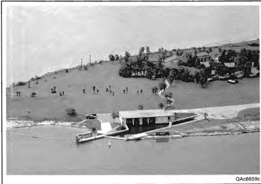
Shoreline along the mainland side of south Laguna Madre characterized by riprap and bulkheads. These features are among approximately 20 shoreline types that are classified in terms of their sensitivity to oil impacts and the relative difficulty of cleanup activities. Marshes and mangroves are ranked the highest in terms of their sensitivity to environmental damage. Photo by William A. White.
