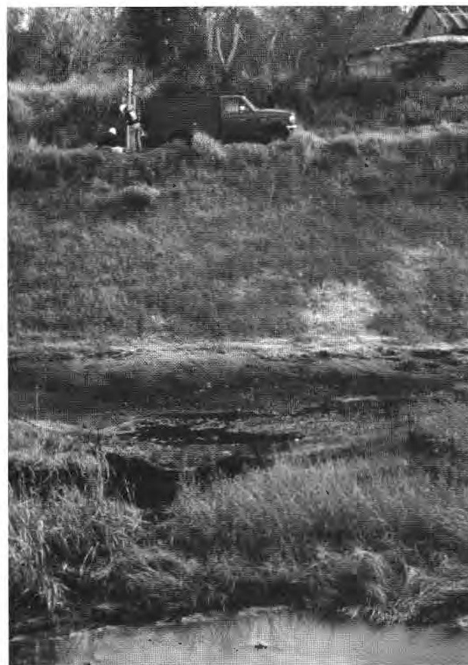
A soil-gas survey was used to delineate the probable extent of a subsurface crude-oil plume in an abandoned oil field, target optimal borehole locations for core samples, and help identify the source of the crude-oil seep. Soil-gas samples were collected using a truck-mounted, hydraulic-driven soil probe and analyzed for volatile aromatic and aliphatic compounds onsite using gas chromatography. Photo shows soil-gas samples being collected along the embankment overlooking the oil seep. Photo by David M. Stephens.
