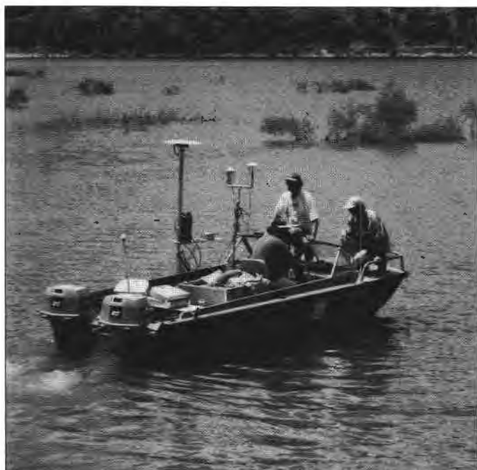
Bureau scientists conducting tests of high-accuracy bathymetric surveying system. Photo by David M. Stephens.
