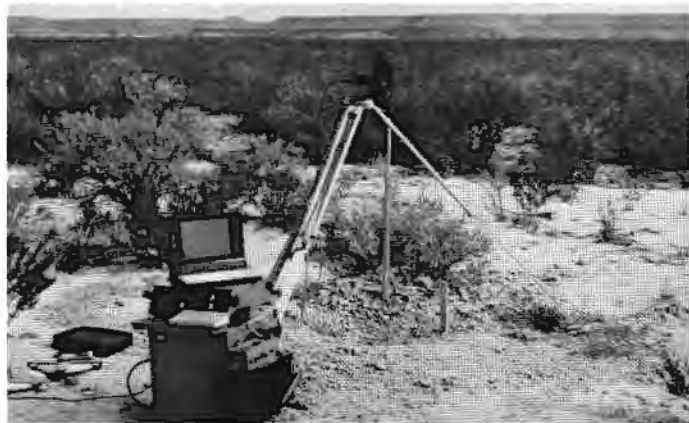
Logging a shallow borehole near Fort Hancock, Texas, using portable gamma-ray and electrical conductivity probes. Resulting logs are used to study changes in soil texture, moisture content, and soil-water chemistry with depth. Photograph by Jeffrey G. Paine.
