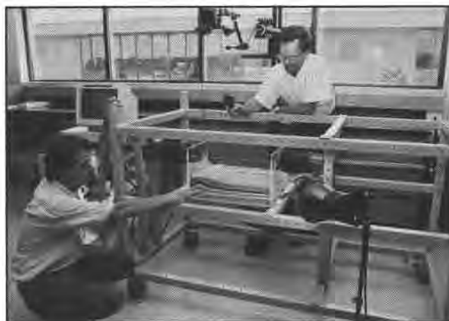
Computer-controlled deformation rig used at the Bureau's Applied Geodynamics Laboratory to deform tectonic models made of layered sand and silicone polymers under a normal-gravity field. Pictured are Bruno Vendeville (left), who designed and constructed the rig, and Martin Jackson, director of the laboratory.
