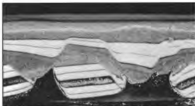
Vertical section through a physical model of diapirs (dark, at bottom) developing during thin-skinned extensional faulting. The shape and location of the modeled diapirs were strongly controlled by faulting in the overburden of stratified sand.
