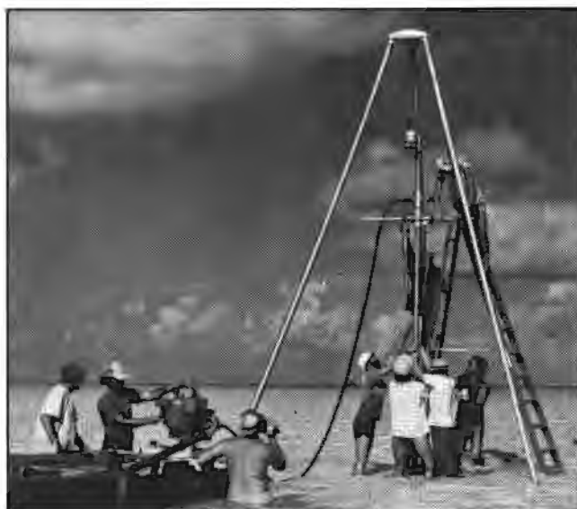
Vibracore drilling rig taking a shallow core of an ooid shoal at Joulter Cays, Bahamas. Such deposits represent a modern analog of major hydrocarbon reservoirs in the Permian Basin.
