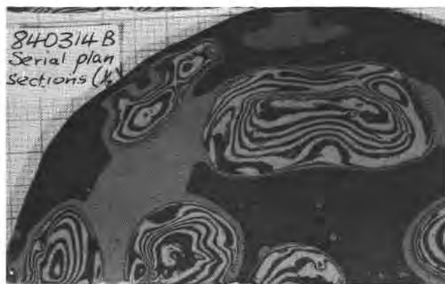
Horizontal section through a centrifuged model showing the internal structure of diapirs. The zebra stripes within the diapirs were originally horizontal and uniformly thick. Experiment performed at the University of Uppsala, Sweden.
