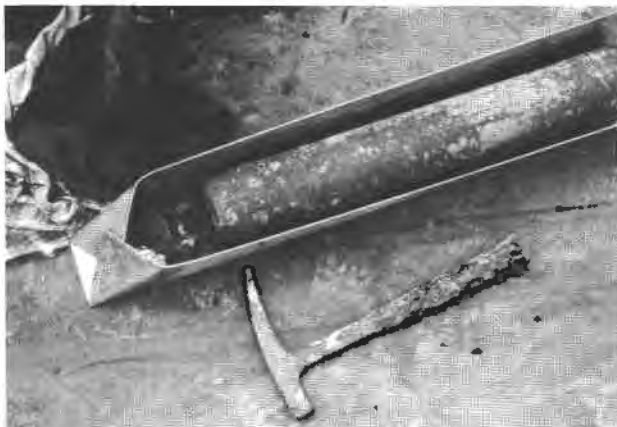
Aligning the orientation equipment as the core barrel is assembled, catching the core in trays on the rig floor, and preliminary examining of core, here showing a conglomerate, for the first Travis Peak well studied in cooperation with an operator on the GRI tight gas sandstone project.
