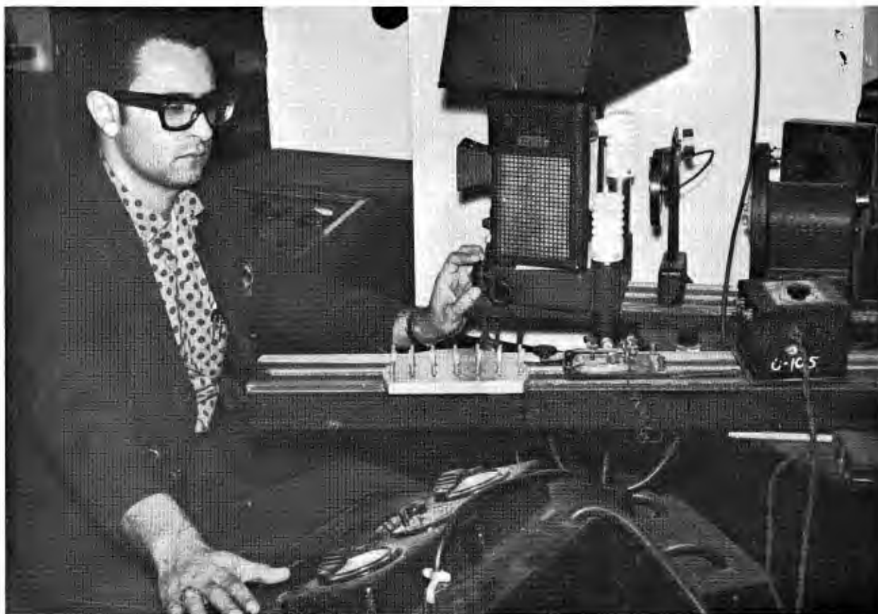
The ARL 1.5 meter emission spectrograph in operation at the Mineral Studies Laboratory. The operator, Fernando D. Cortes, is a chemical engineering student employed as a laboratory assistant by the Bureau.
