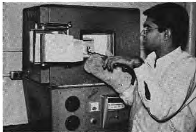
Clay sample undergoing firing tests in the Mineral Studies Laboratory's new LECO high temperature furnace. This furnace will develop temperatures up to 3,000° F and is being used for evaluating potential refractory materials.
