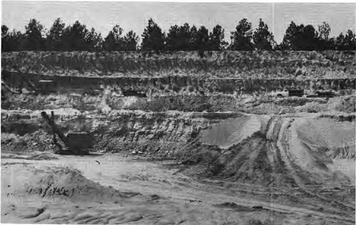
Open-pit, bench mining of bentonitic clay deposits, Bennett-Clark Company pit, southern Angelina County. Bentonitic clays mined in east Texas are used primarily as rotary drilling muds, filtering and decolorizing materials, and insecticide and fungicide fillers.
